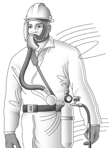
Tight-fitting Atmosphere-Supplying Respirator with an auxiliary escape bottle APF=10,000 in escape mode only; otherwise APF=1,000 Full facepiece Needs to be fit tested
