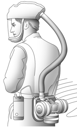
Loose-Fitting Powered Air-Purifying Respirator (PAPR) APF=25
