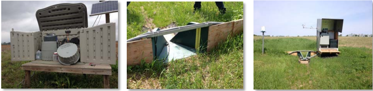
Image 8. Edge-of-field monitoring in practice. The pictures on the left and in the center show monitoring stations that allow NRCS to measure the amount of nutrients and sediment in water at the edge of a farm field. The picture on the right is of a calibrated flume used by USGS to measure water flow and loading of nutrients and sediment. (Credit: USDA/NRCS.)
