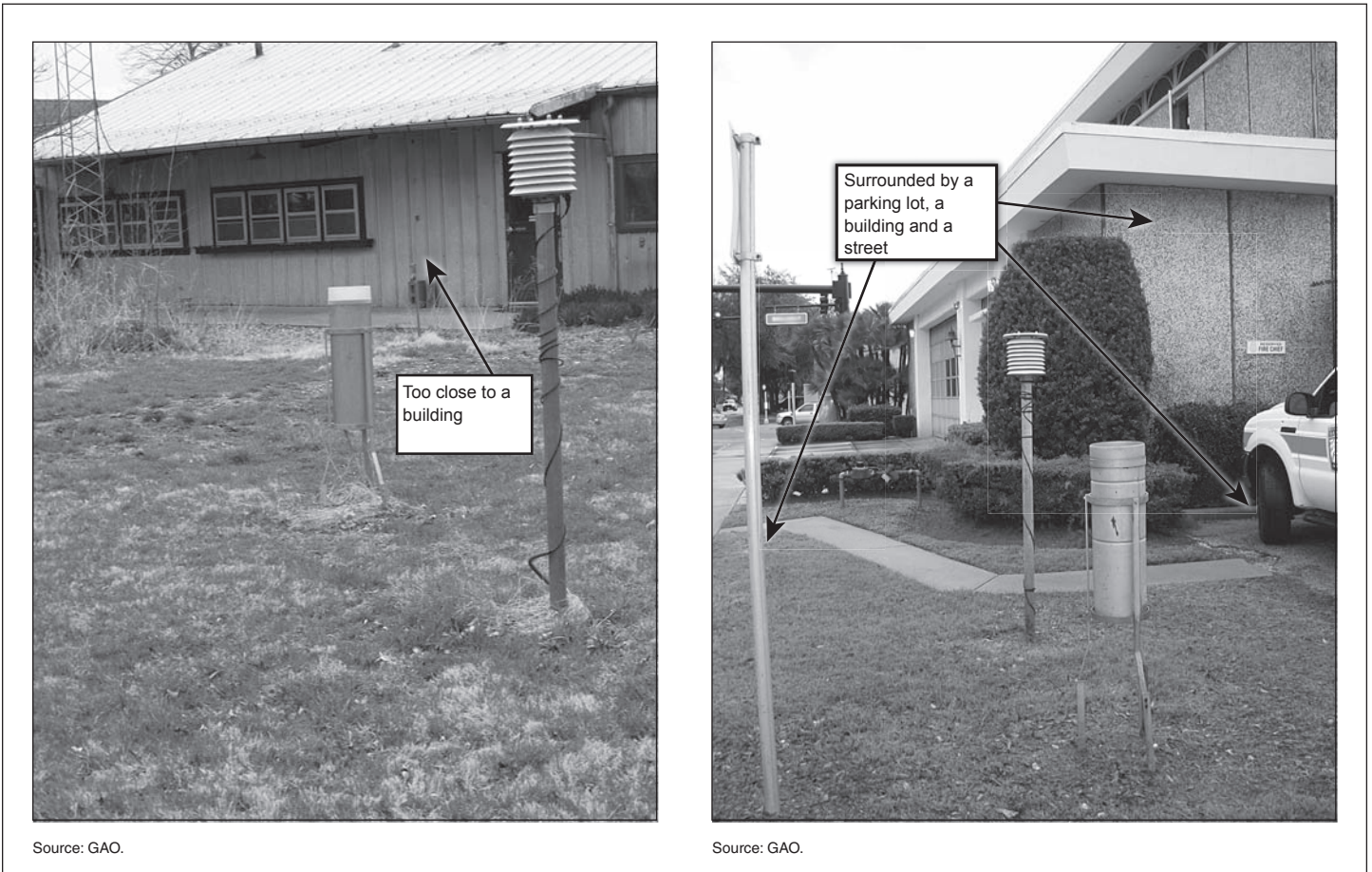
Figure 4: Comparison of Conditions at Two USHCN Stations That Do Not Meet NWS Siting Standards
