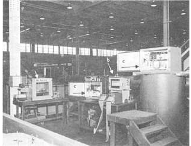
Figure 17. Laboratory evaluation of control components. (a) environmental chamber, (b) data acquisition equipment, (c) automatic control components. Photo P801-D-73320
