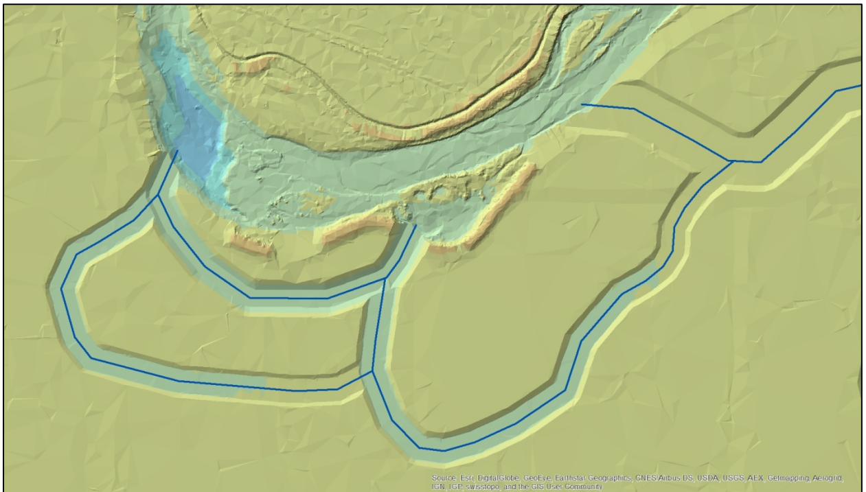
Figure 5. Final terrain with channel cuts.
