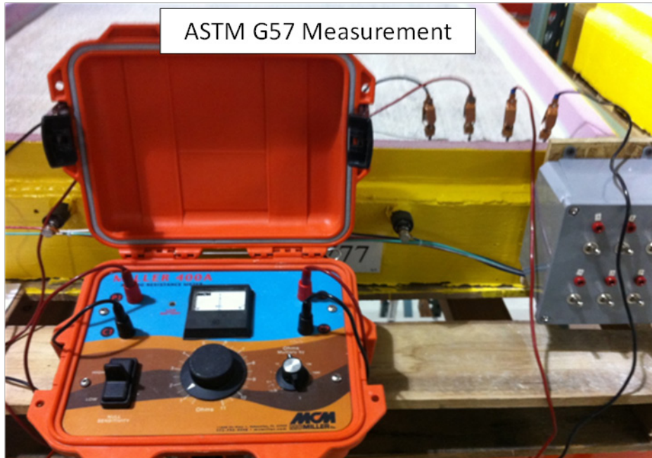
Figure 14 – Example for measuring electrical resistivity according to ASTM G 57 using the resistivity electrodes.
