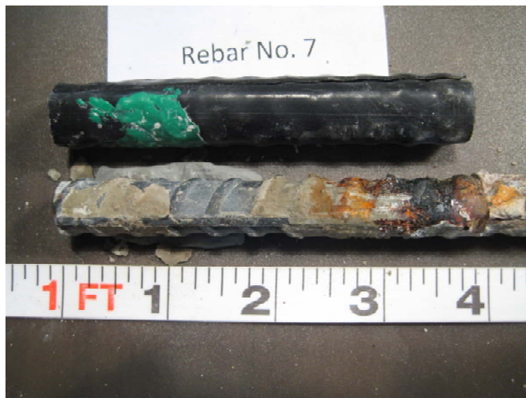
Figure 139 – Corrosion observed underneath CN paste/shrink tube end coating
