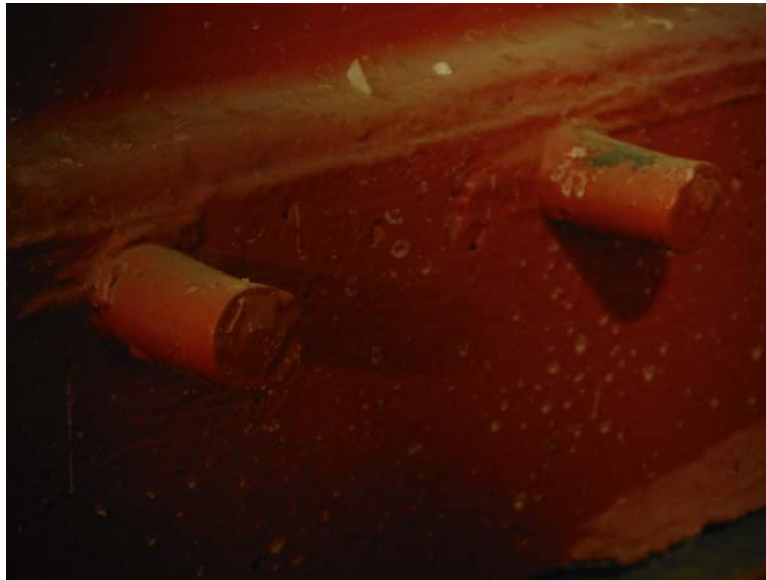
Figure 66 - Photograph of batch #5 reinforcing bar end treatment
