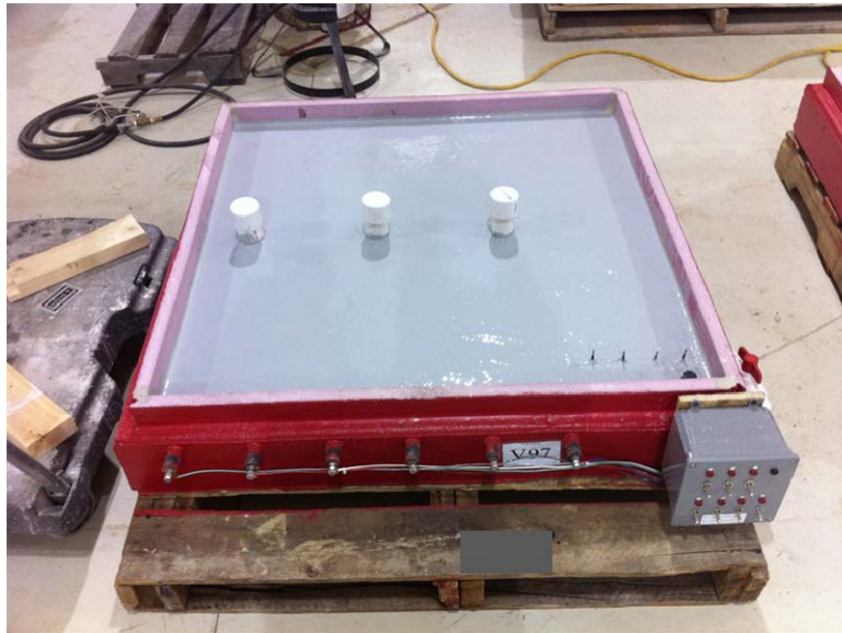
Figure 113 – Completed application of base coat
