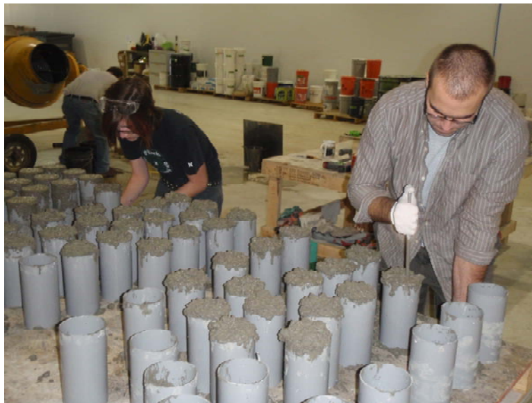
Figure 95 – Casting cylinders for concrete characterization
