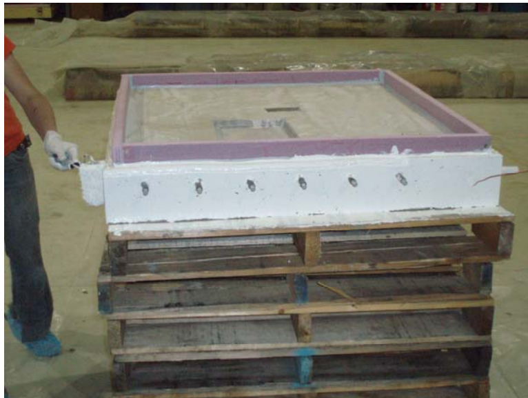
Figure 88 - Application of Epoxy to Test Specimen
