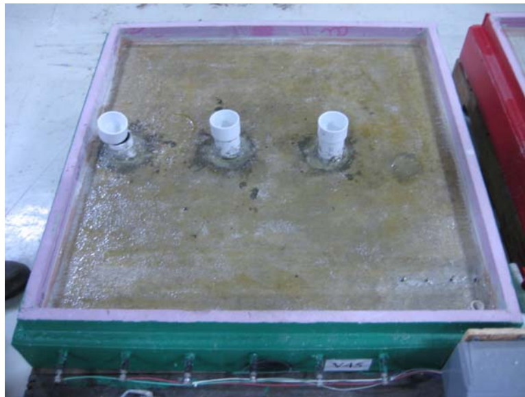
Figure 111 – Completed application of primer
