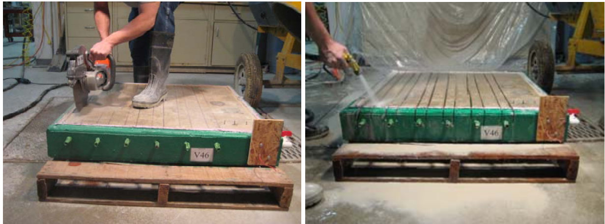
Figure 130 – Cut parallel to rebar
