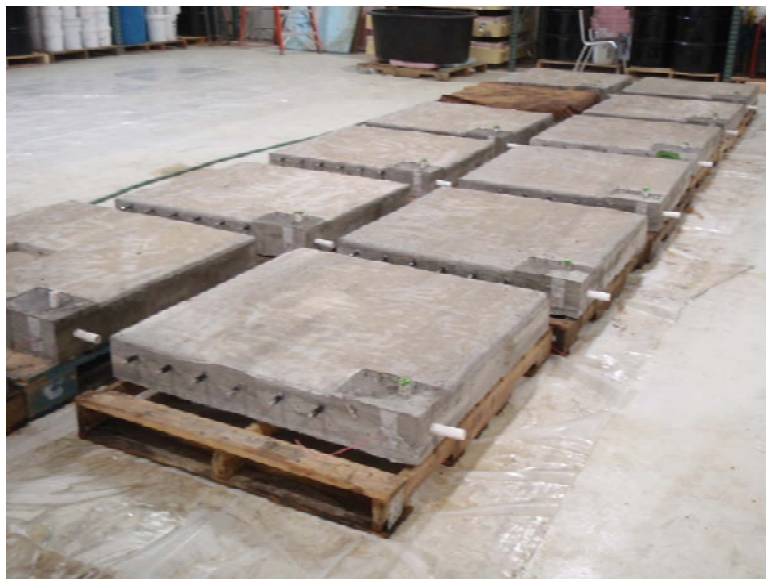
Figure 86 – Test specimens after form removal
