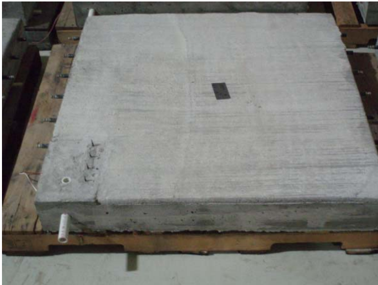
Figure 84 – Completed slab with resistivity pins
