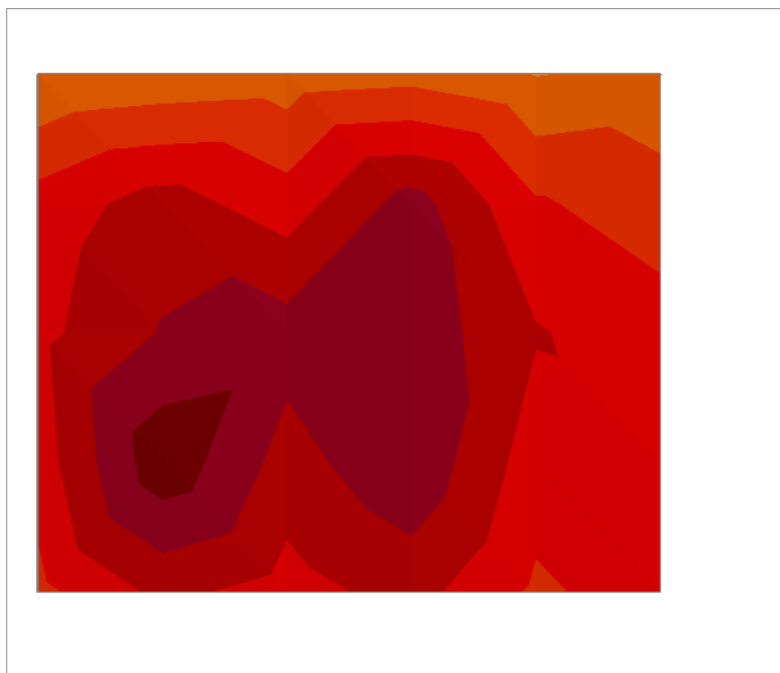
Figure 180 - Half-cell potential mapping prior to destructive analysis, slab #91 - Control
