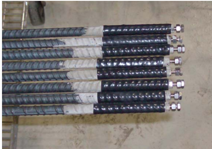
Figure 63 – Rubber Tubing Shrink Wrapped on to End of Reinforcement Bar
