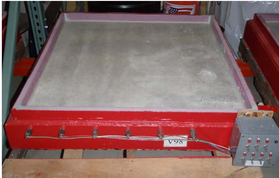
Figure 60 – Completed Batch #5 Topical Treatment Test Specimen
