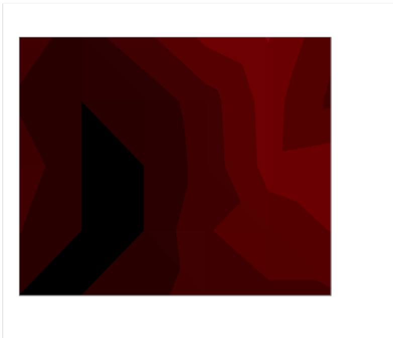
Figure 170 - Half-cell potential mapping prior to destructive analysis, slab #72 - Control
