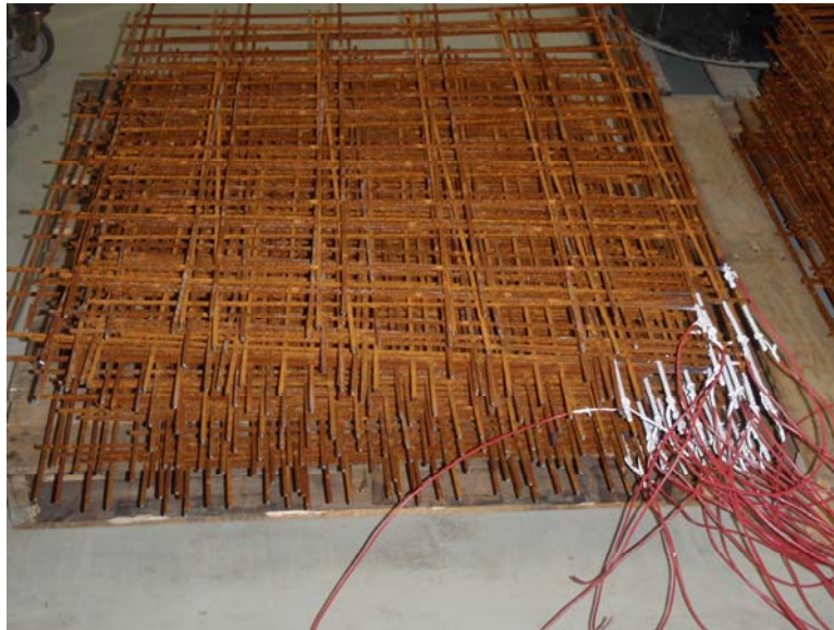
Figure 68 - Stack of Weld Wire Form Sheets with Installed Electrical Leads
