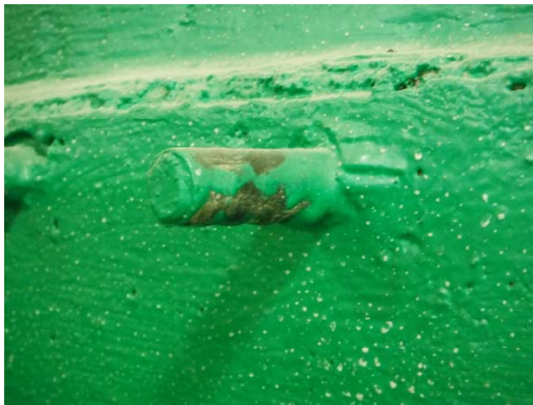
Figure 64 – Photograph of batch #3 reinforcing bar end treatment
