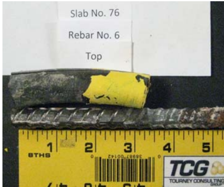
Figure 140 – H 2 SO 4 Pickle/Epoxy end treatment with no visual signs of corrosion
