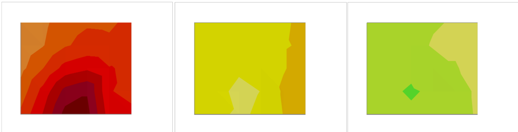
Figure 44 – Half-cell potential mapping over time, prior to repair, after 5 ponding cycles, and after 8 ponding cycles (Sealer)
