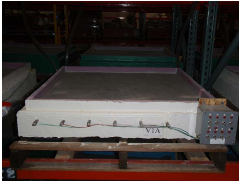
Figure 92 - Test Specimen with Completed Wiring and Junction Box
