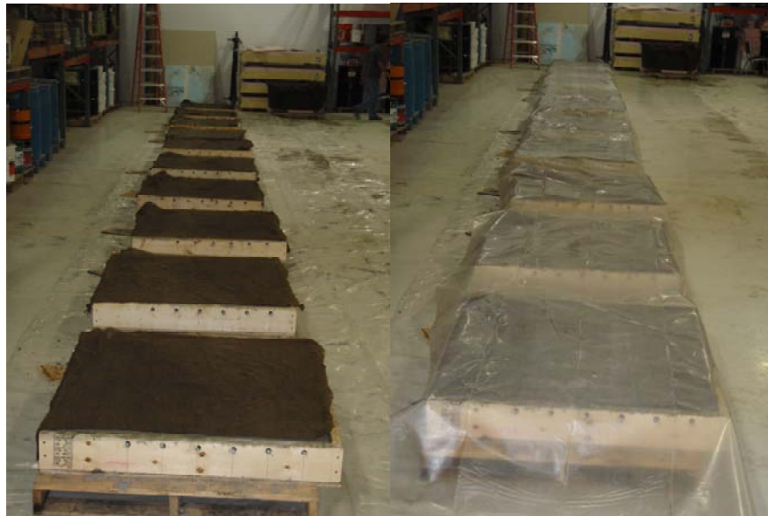
Figure 85 - Test specimens covered with burlap and plastic
