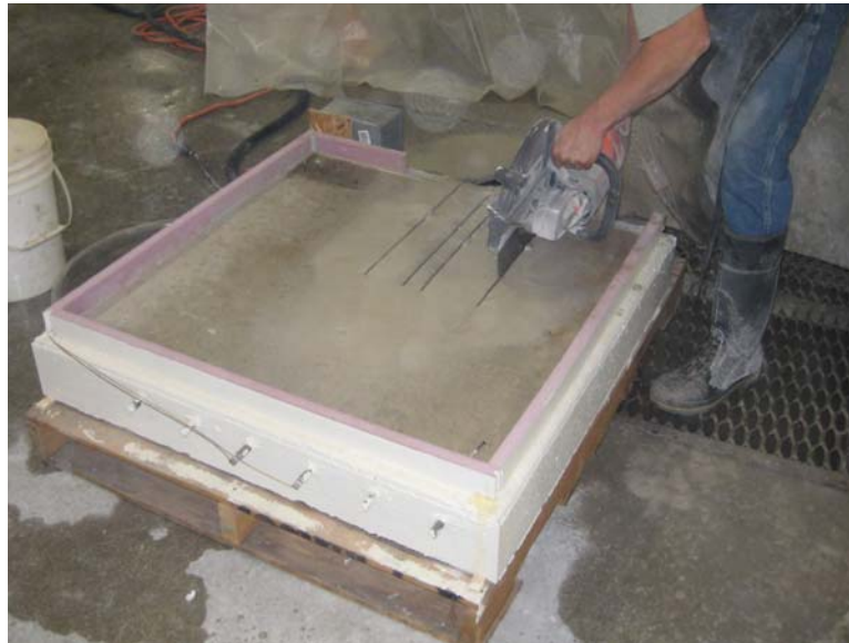
Figure 118 – Saw cut and chip out concrete in hotspot area
