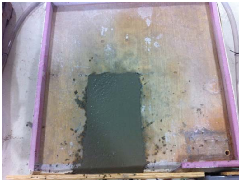
Figure 124 – Slab with completed repair mixture treatment
