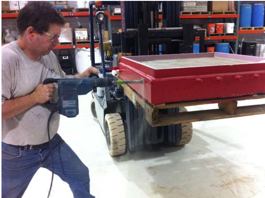
Figure 100 – Installation of internal relative humidity and temperature ports
