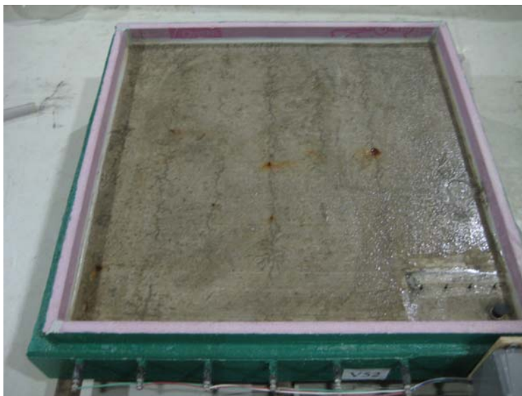
Figure 105 – Slab with completed application of 40% silane sealer
