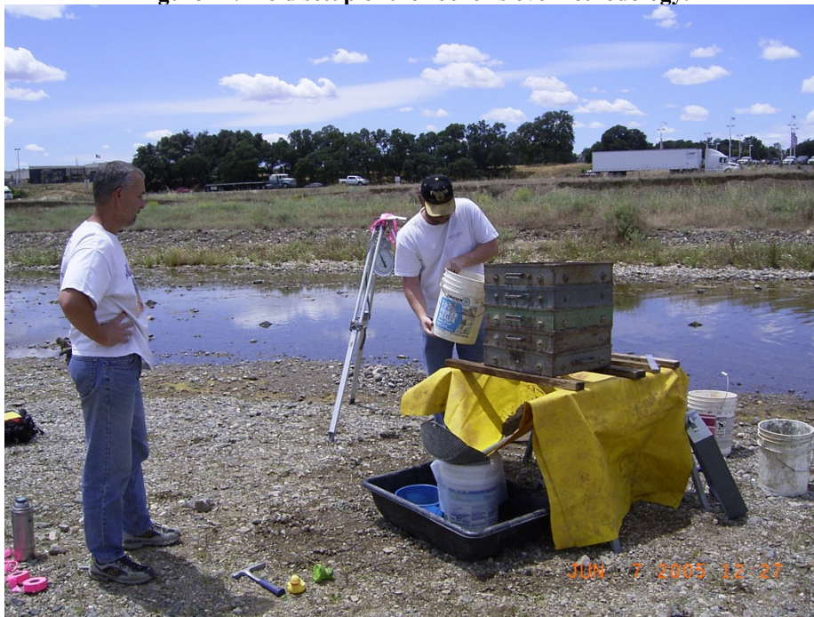
Figure 12. Alternative field sieving setup involving large sieves.
