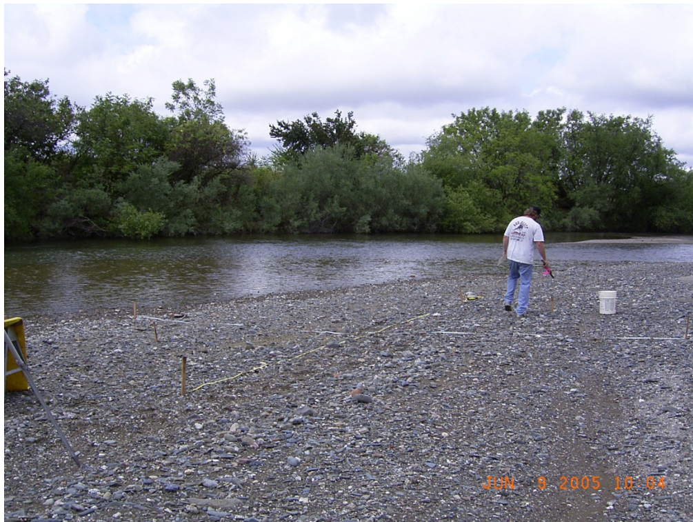
Figure 8. Photograph of grid used to collect Wolman pebble count at Elder Creek.
