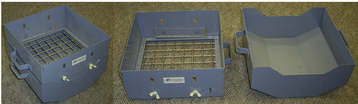
Figure 10. Rocker sieve used for on-site sieving.
