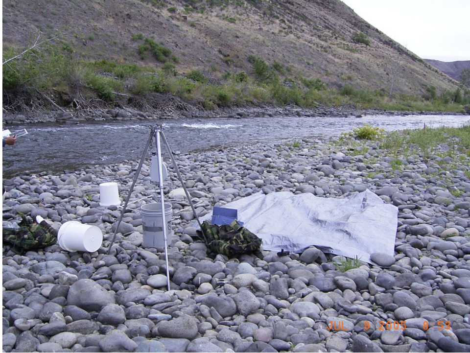
Figure 11. Field setup of the rocker sieve methodology.
