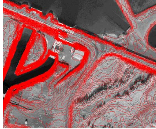
Fig. 39. An orthophoto view of the Dam at Dry Falls. Fig. 40. LIDAR generated elevation contours at 1' resolution.
