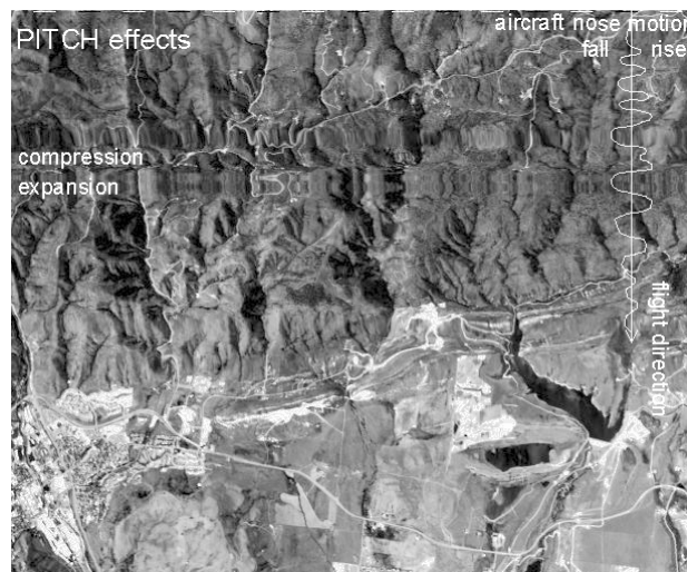
Fig. 52. Distortions in caused by pitch.
