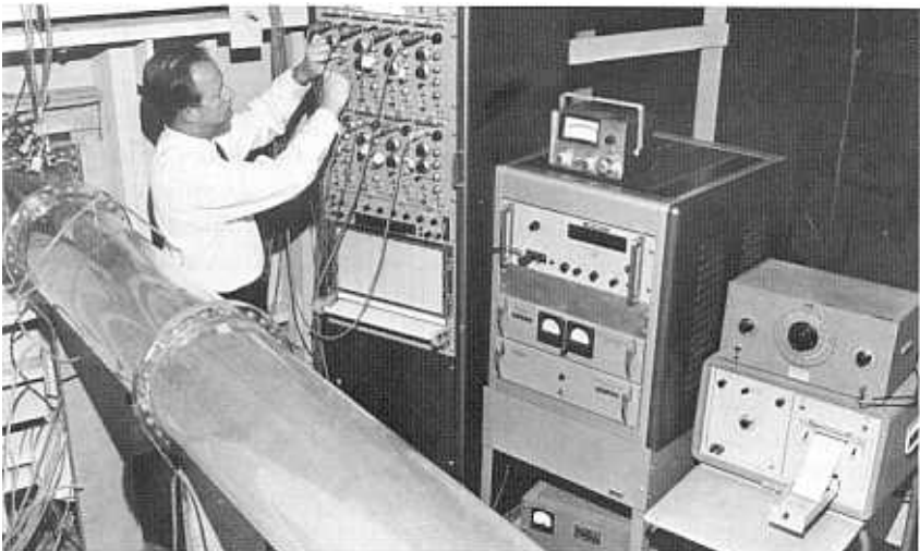
B. Measuring pressure fluctuations near entrance to penstock model. PX-D-58747
