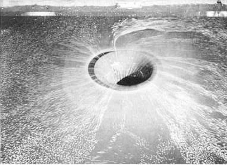
A. Free-flow crest at partial discharge. (Paper confetti on water surface for detecting flow patterns and determining velocities.) P805-D-46309NA
