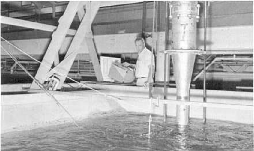
Figure 2-6.—Wave measurement with capacitance-wire transducers. PX-D-63963
