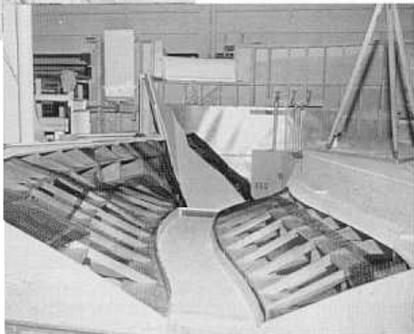
Figure 4.2.—Stages in constructing an arch dam spillway model.
