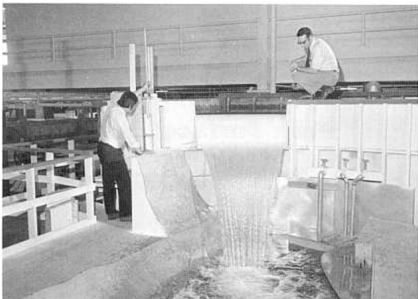
Figure 5-1.—Overfall spillway and plunge-type stilling basin. P801-D-79224
