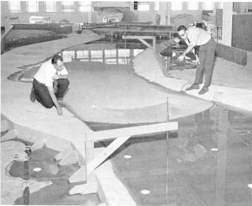
Figure 6-4.—Fixed-bed model of river for study of booms used to control location of ice jams. P801-D-79244
