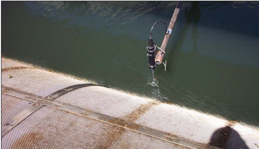
Figure 27. A cantilevered steel mount with a horizontally adjustable arm was used to measure velocities close to the screen face near the surface (as shown) and under the curvature of the screen (DeMoyer, 2004).
