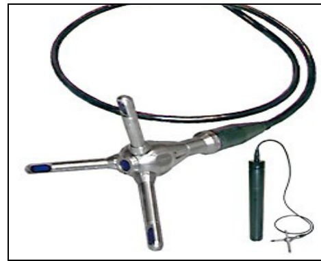
Figure 12. Nortek Vector velocimeter 6-MHz probe and submersible signal processing housing (photo courtesy of Nortek).
