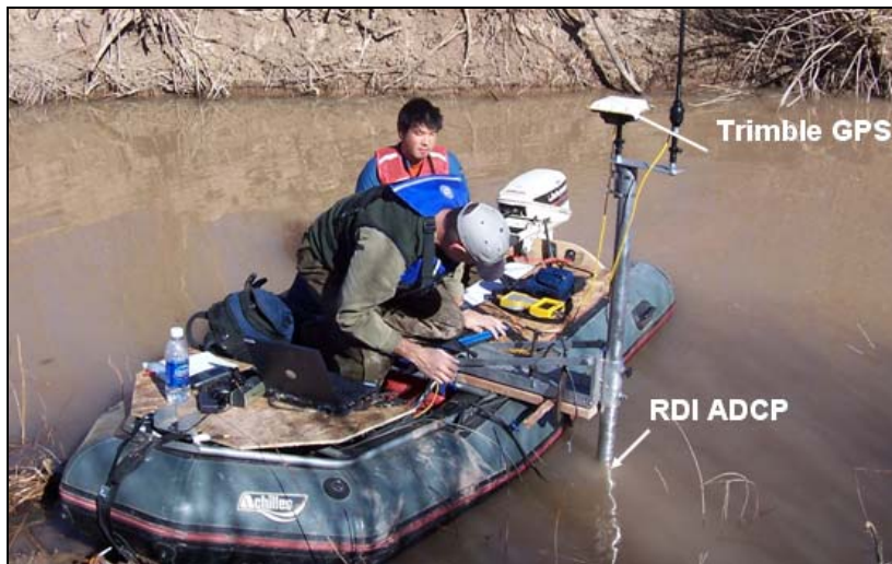
Figure 22. A typical setup using a Teledyne/RDI Workhorse Rio Grande ADCP with Trimble GPS to collect bathymetric survey data.
