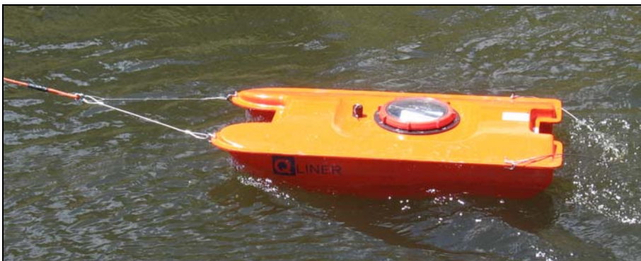
Figure 19. OTT Qliner acoustic Doppler profiler (photo courtesy of OTT).
