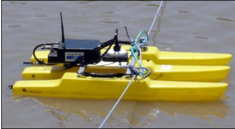
Figure 20. SonTek/YSI RiverCat acoustic Doppler profiling system (photo courtesy of SonTek/YSI).
