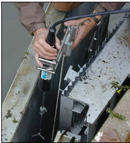
Figure 33. Mounting an ADV to the louver line.
