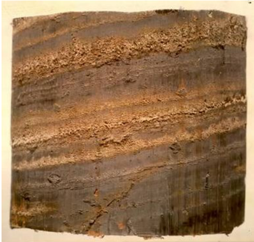
Figure 60. —A sample of material taken in the slide area of the canal. The material is clay with sand lenses.
