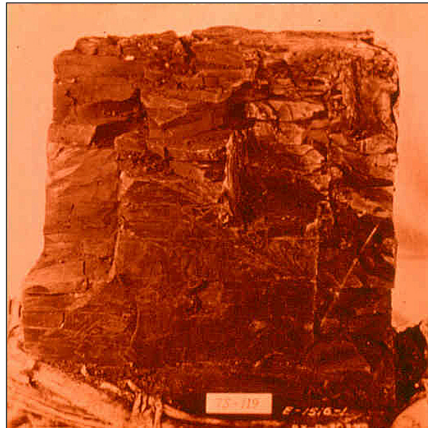
Figure 54. —A block sample of fresh shale allowed to air slake.
