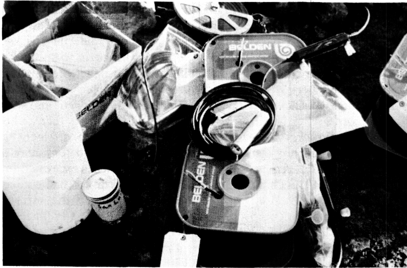
Figure 2-27.—Vibrating-wire piezometer equipment. P801-D-81010.
