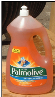
Figure 12. —Dish soap used to simulate slippery invert conditions.
