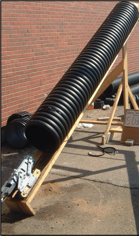
Figure 20. —VersaTrax 150 system traveling up a 30-degree dry invert slope.
