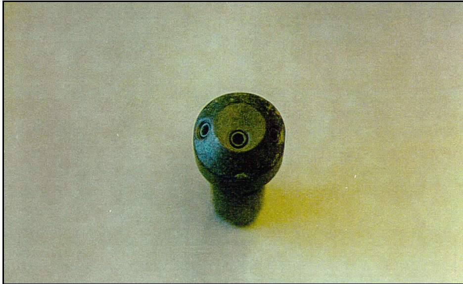
Figure 33. —Front view of the rotating cleaning head, showing the opposing side jets pointing forward at 45° and the offset front jet pointing forward at 10°.
