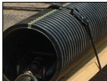
Figure 11.—Bungee cords used to secure the pipe to the testing apparatus.
