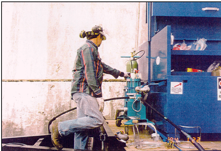
Figure 29. —Driller adjusting the pressure regulator between the high pressure pump and the delivery lines supplying water to the control.
