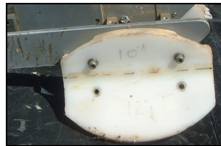
Figure 18. —Stabilization wings used on the MiniTrac system.
