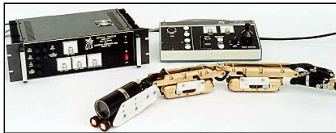
Figure 2.—RCVI instrumentation and control equipment.
