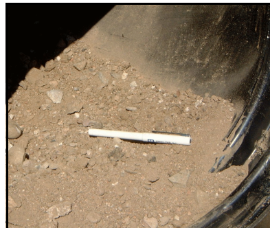
Figure 13. —Random mixture of fine and coarse aggregates used to simulate sediment deposition on the pipe invert.
