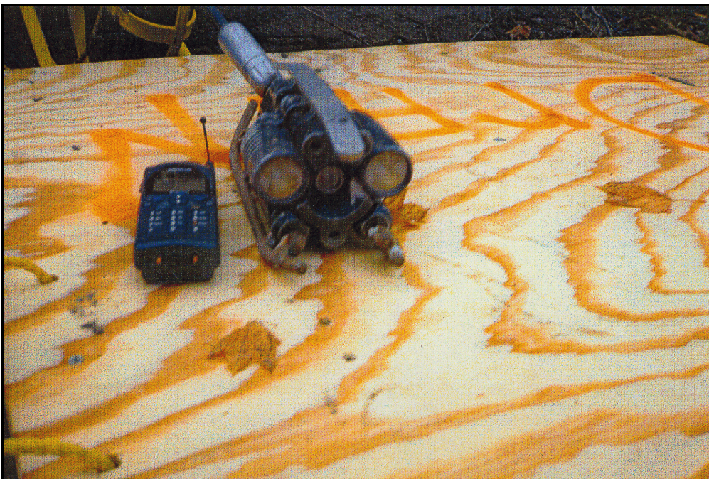
Figure 67.—Sled-mounted camera (the cell phone provides scale).
