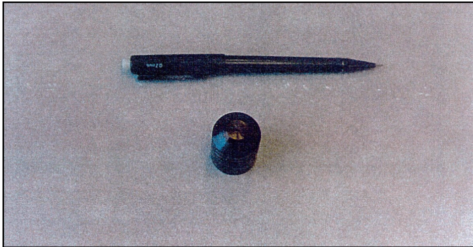
Figure 34. —Front view of nonrotating sewer cleaning nozzle. One predrilled hole points straight forward from the center. Three other predrilled evenly spaced holes point straight forward from the beveled portion. This cleaning head is used for flushing with pressures of less than 2,000 lb/in 2 .
