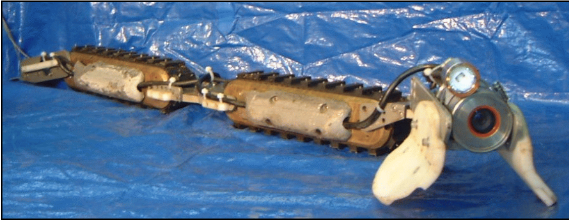
Figure 8. —The MiniTrac remotely controlled inspection system.
