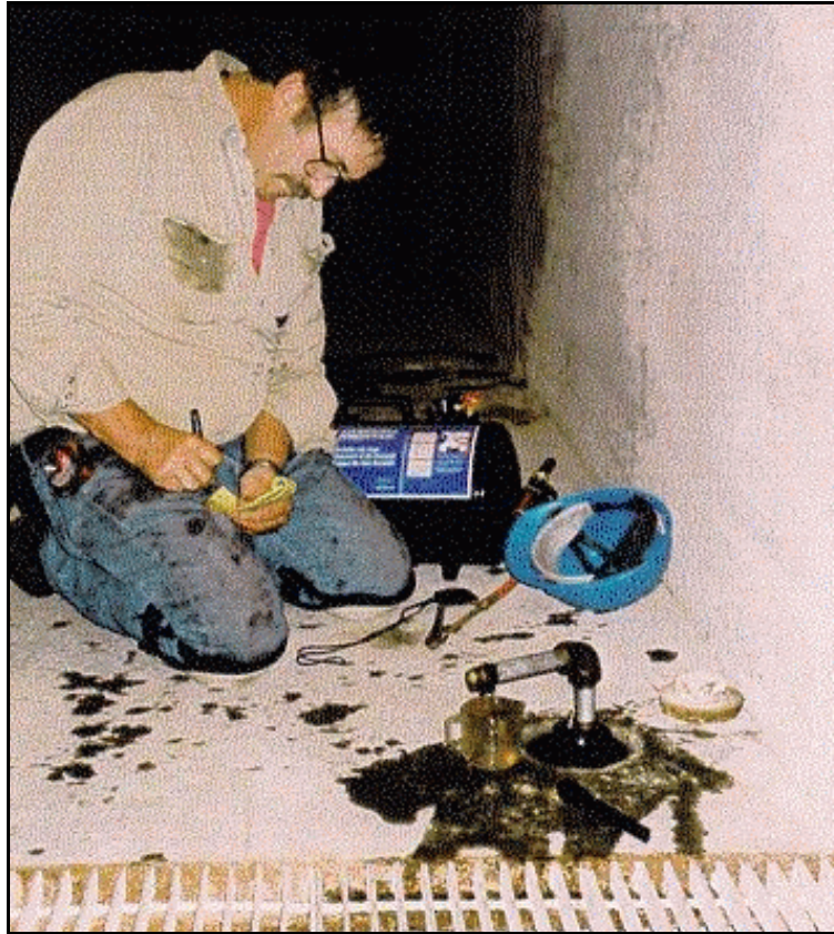
Figure 40.—Individual drain flow measurement being recorded.
