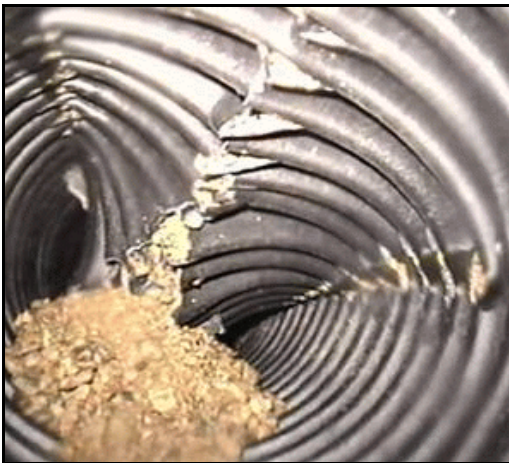
Figure 100. —HDPE pipe experiencing failure at the crown. Materials surrounding the pipe have entered through the failure.
