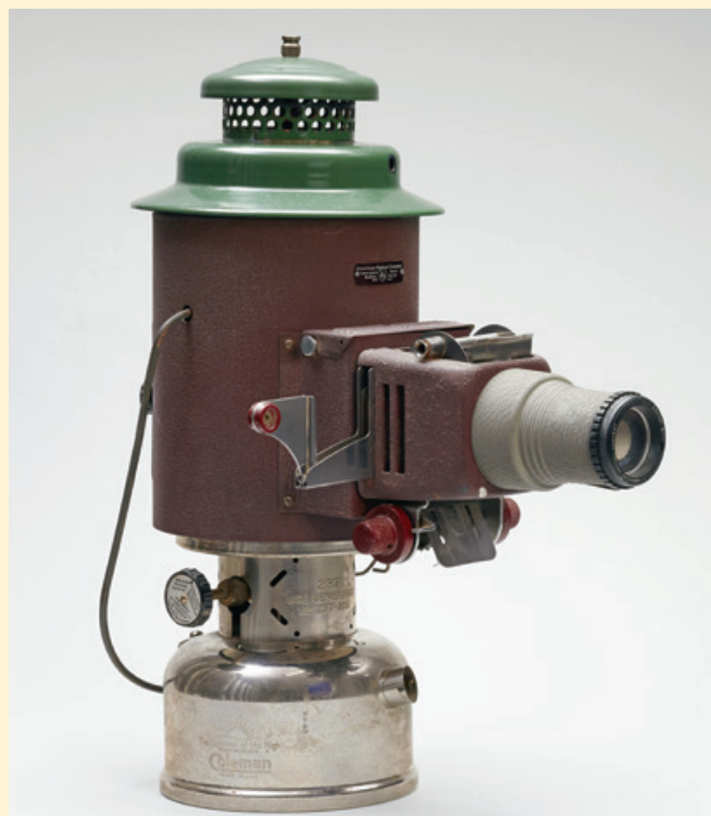
A 1950s kerosene-powered slide projector from the U.S. Embassy in Singapore. Diplomats used it to show slides or film strips in areas with limited or no electricity. Department of State
