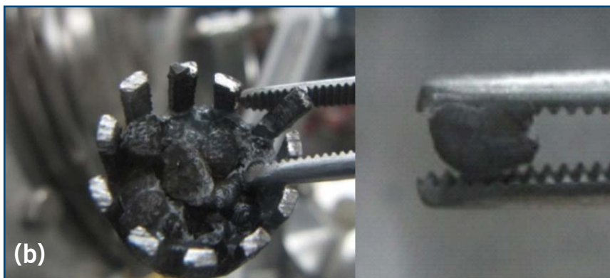
Figure 2. Photograph of U_3O_8 granules.
