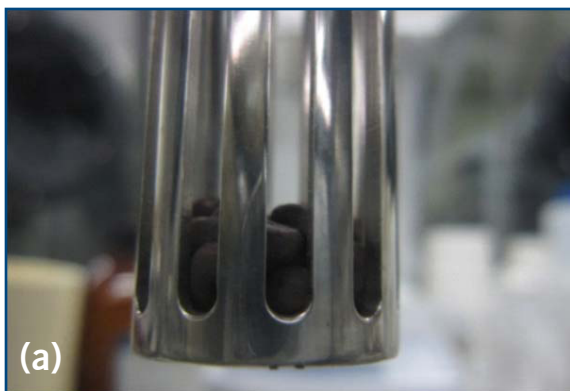
Figure 3. U_3O_8 granules (a) before and (b) after electro-reduction testing.
