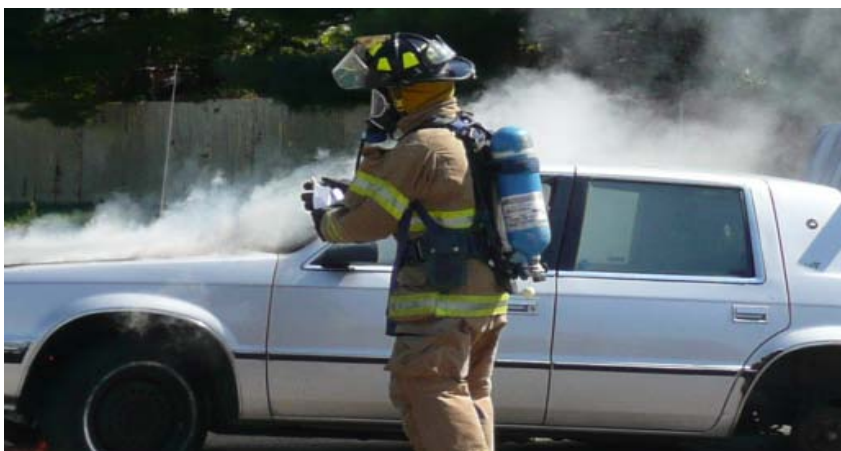
Figure 4. Fire fighter using Summa canisters to sample VOCs from a vehicle fire.
