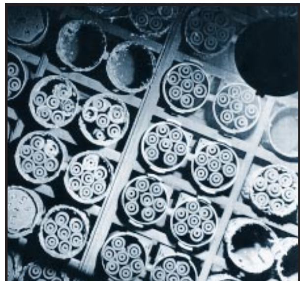
Corroding spent-fuel elements from the Hanford N Reactor are stored in an unlined concrete pool in the 105 K-East area. Corrosion releases radioactive materials to pool water, posing a hazard to workers. Hanford Site, Washington.
