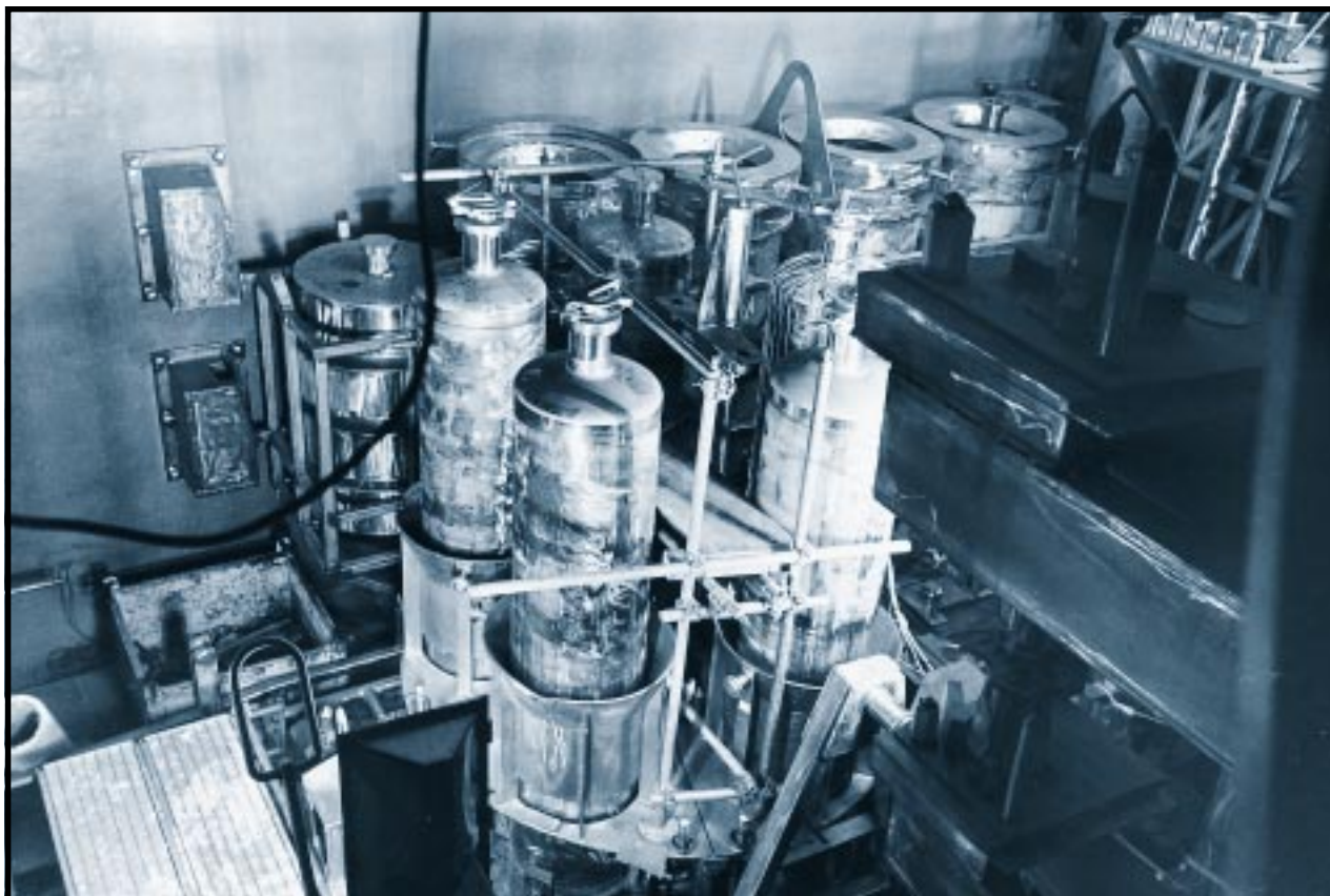
These stainless-steel canisters weigh 1,100 pounds each. When full of vitrified waste, they will weigh 3,700 pounds each and will be extremely radioactive. Defense Waste Processing Facility, Savannah River Site, South Carolina. June 15, 1993.
