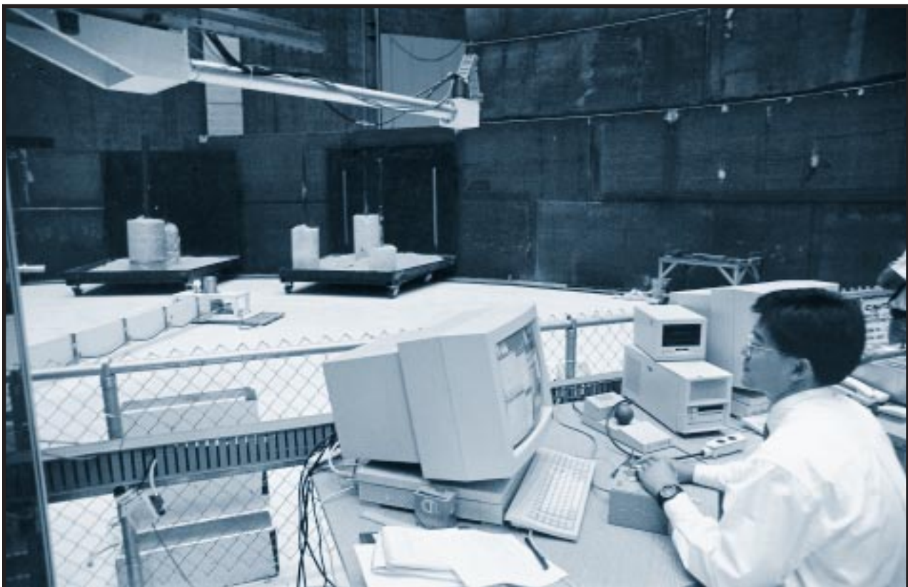
Advanced robotics for cleanup of high-level waste are demonstrated by research scientist Jae Lew. The robotic manipulator in the distance is designed to break up and remove sludge and solidified waste inside a high-level-waste tank. This system is also used to develop, test, and evaluate a variety of methods for the retrieval of high-level waste. 337 Building, Hanford Site, Washington. July 11, 1994.
