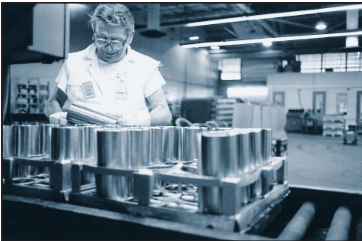
Final inspection of uranium “billets.” These billets of depleted uranium metal were produced at the Fernald Plant to be used as the cores of Mark 31 targets. Jack Schick, a metals worker, conducts a final inspection of a new batch before shipping them to the Savannah River Site, where they would be clad in aluminum, bombarded with neutrons, and partly transformed into plutonium. Plant 6, Fernald Feed Materials Production Center, Fernald, Ohio. December 17, 1985.
