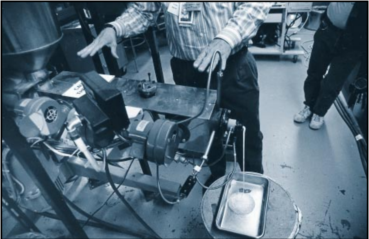
The encapsulation of low-level mixed waste in polyethylene is an innovative waste-handling technology in a pilot phase at Rocky Flats. A heated stream of recycled polyethylene is combined with simulated low-level mixed radioactive waste, encapsulating each particle of waste as the mix is poured into molds. Building 881, Rocky Flats Plant, Colorado. March 21, 1994.
