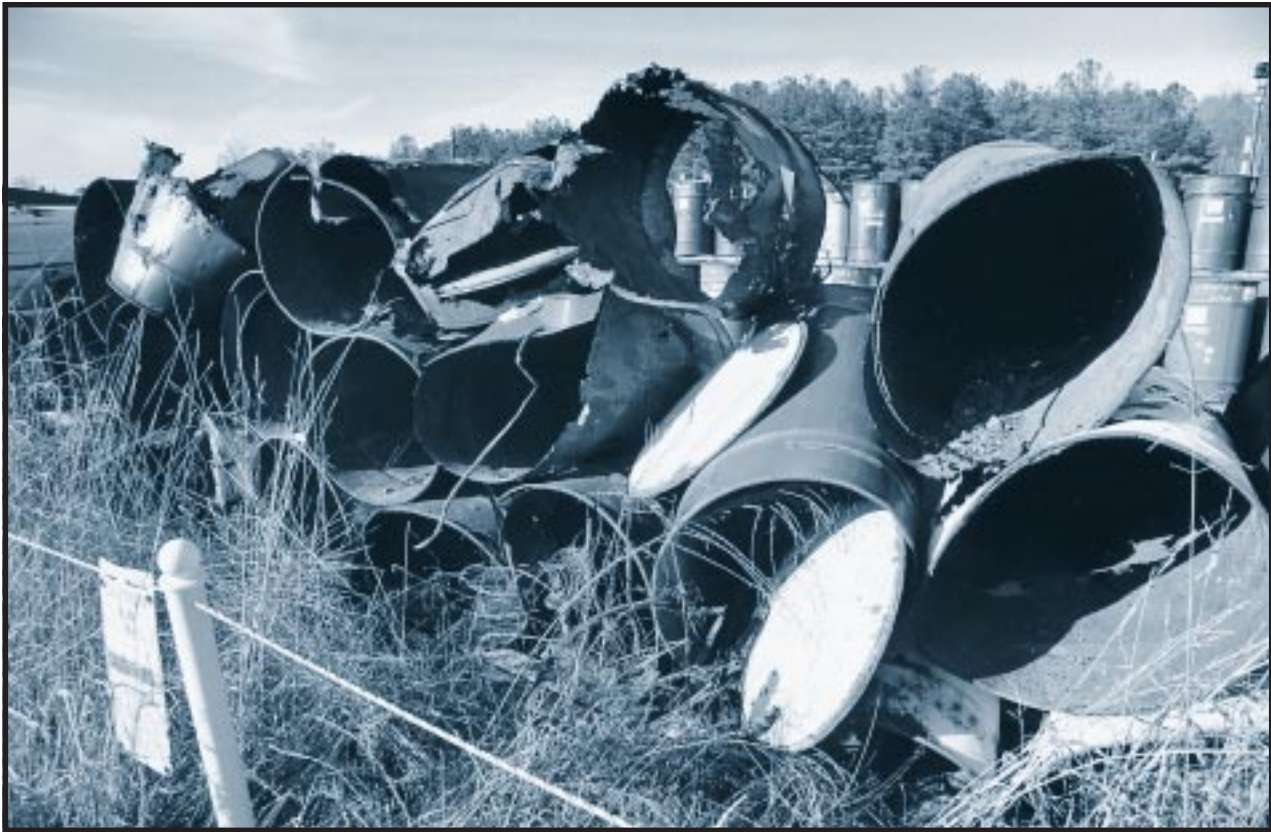
Empty drums used for storing waste await treatment and disposal at Oak Ridge. These drums corroded prematurely when a 1987 waste-stabilization project failed to follow guidelines for combining waste sludge with cement. K-1417 Drum Storage Yards, Pond Waste Management Project, Oak Ridge, Tennessee. January 10, 1994.
