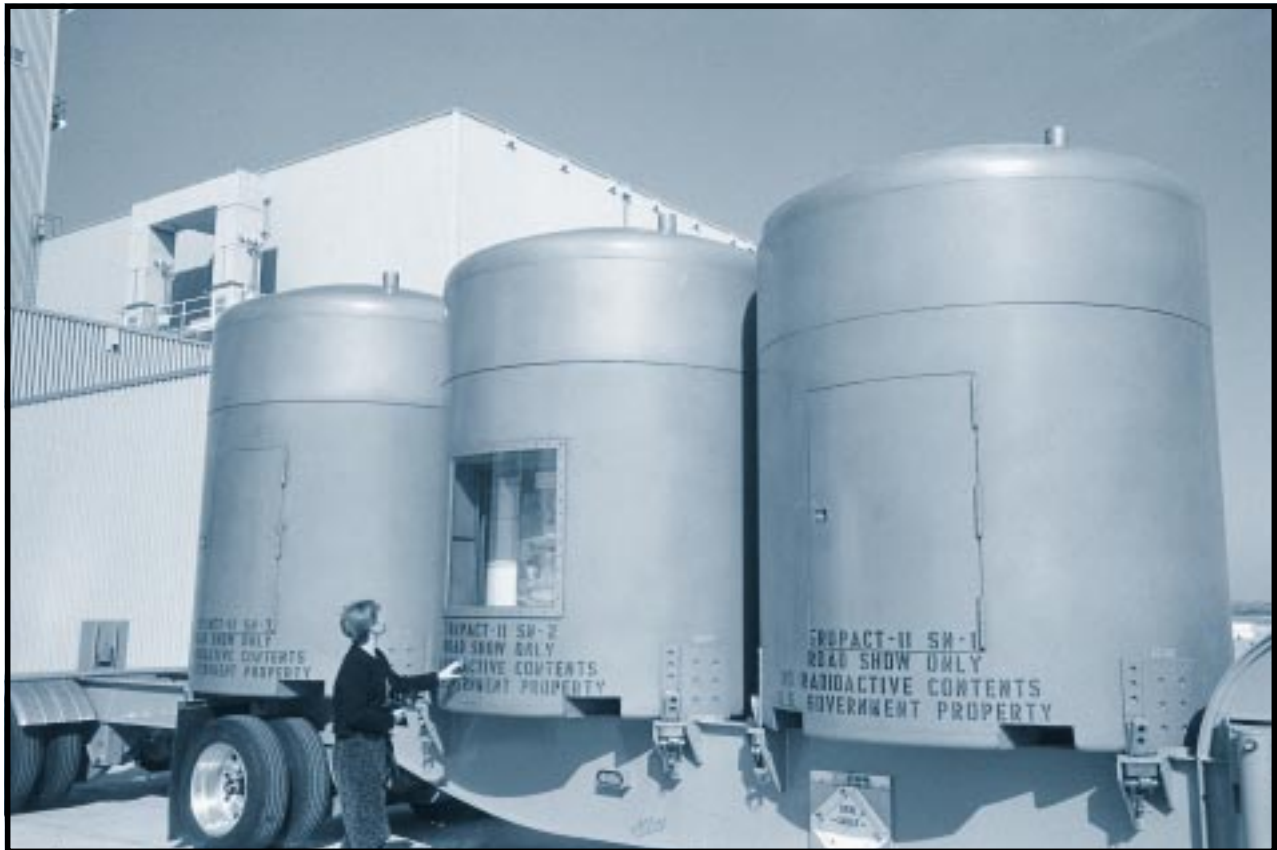
Demonstration models of special casks for shipping transuranic waste show how transuranic wastes will be trucked cross-country to the Waste Isolation Pilot Plant. Each of these TRUPACT-II (Transuranic Package Transporter) casks can hold fourteen 55-gallon drums. A window in the center cask displays mock waste drums cut open to reveal typical constituents of transuranic waste. This “roadshow” flatbed unit is used for public education and for training emergency-response teams along planned waste-shipment routes. Waste Isolation Pilot Plant, near Carlsbad, New Mexico. February 25, 1994.
