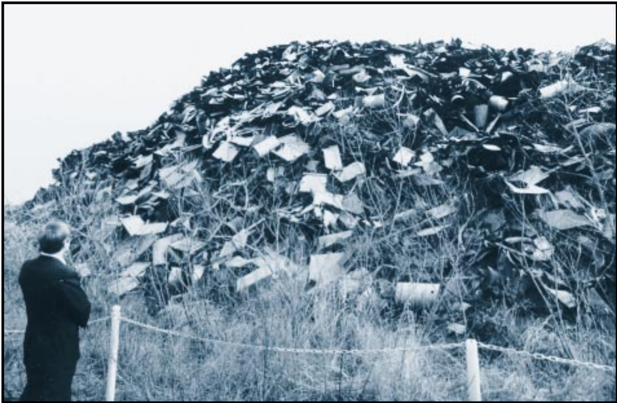
This yard for contaminated scrap metal contains heaps of slightly radioactive scrap steel, ferrous metal, and nickel-plated metal left over from upgrades and renovations to the K-25 Gaseous Diffusion Plant at Oak Ridge over the years. K-25 Scrapyard, Oak Ridge, Tennessee. January 10, 1994.
