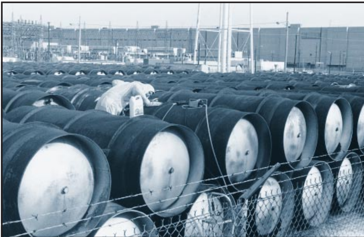
Uranium hexafluoride cylinders are stored near the K-25 Gaseous Diffusion Plant. Each cylinder contains 10 to 14 tons of depleted uranium hexafluoride. The K-25 plant stores about 5,000 of these cylinders, some of them 40 years old. Here, a worker is using ultrasound to evaluate the effects of external corrosion on a steel cylinder. Cylinders closest to the ground can experience accelerated corrosion. K-1066K Cylinder Storage Yard, K-25 Site, Oak Ridge, Tennessee. January 9, 1994.
