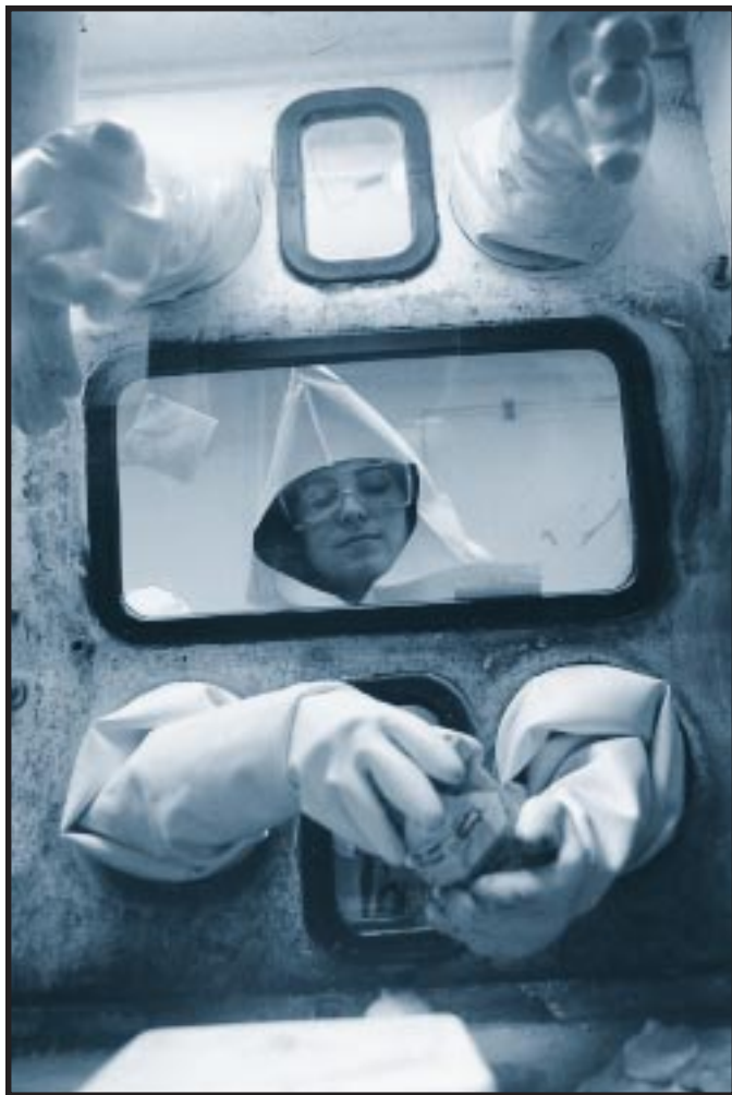
Calibration spheres like this one surveyed by Y-12 machinist Danny Bush were used to set instruments that check the manufacturing specifications for weapons parts. Crucial components of nuclear warheads must be accurately shaped to within a few millionths of an inch. Y-12 Metrology Laboratory, User Facility Skills Demonstration Center, Y-12 Plant, Oak Ridge, Tennessee. January 12, 1994.
