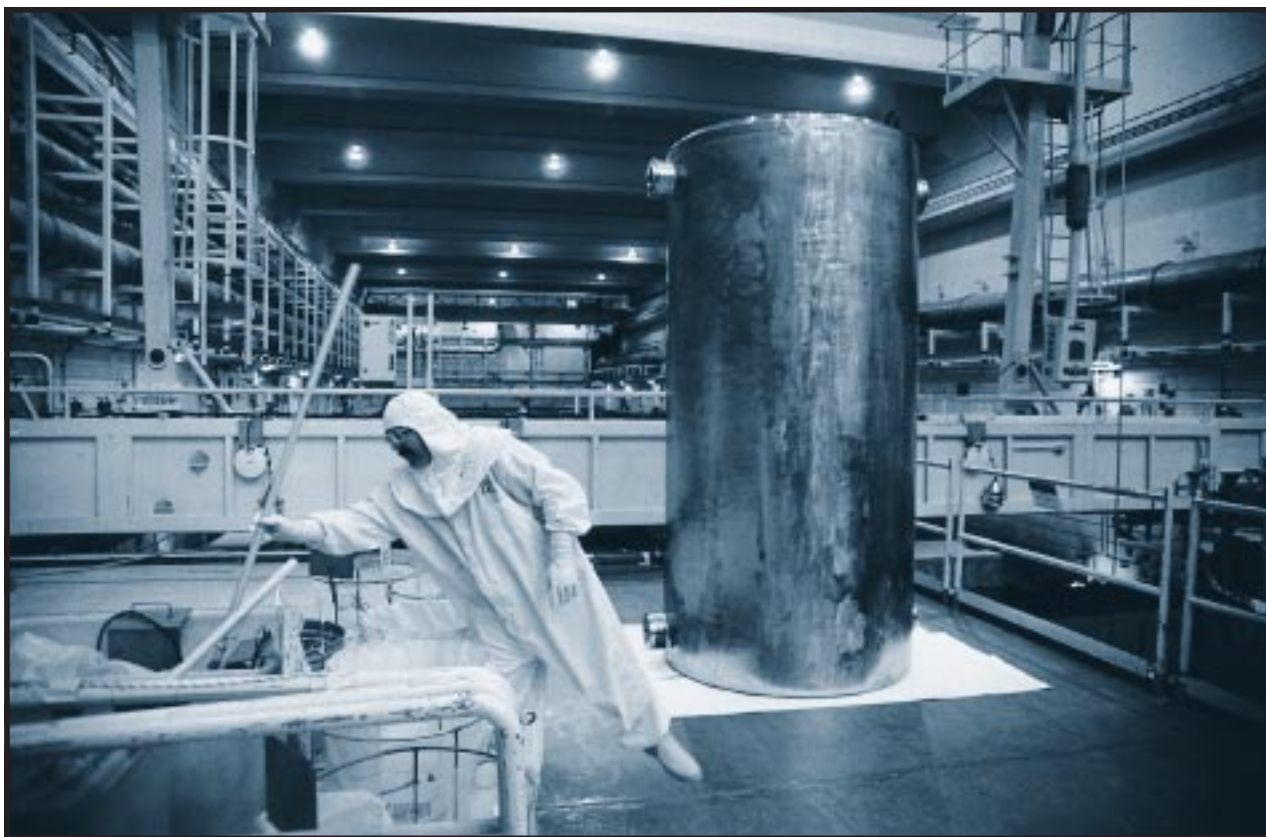
A cask for shipping spent fuel stands empty after its cargo of irradiated nuclear fuel has been deposited into the nearby spent-fuel pool for storage. A worker is completing decontamination of the cask so that it can be reused. The spent-fuel pool in the background holds 22 million gallons of water. Idaho Chemical Processing Plant, Fuel Storage and Treatment Facility, Building 666, Idaho National Engineering Laboratory. March 17, 1994.
