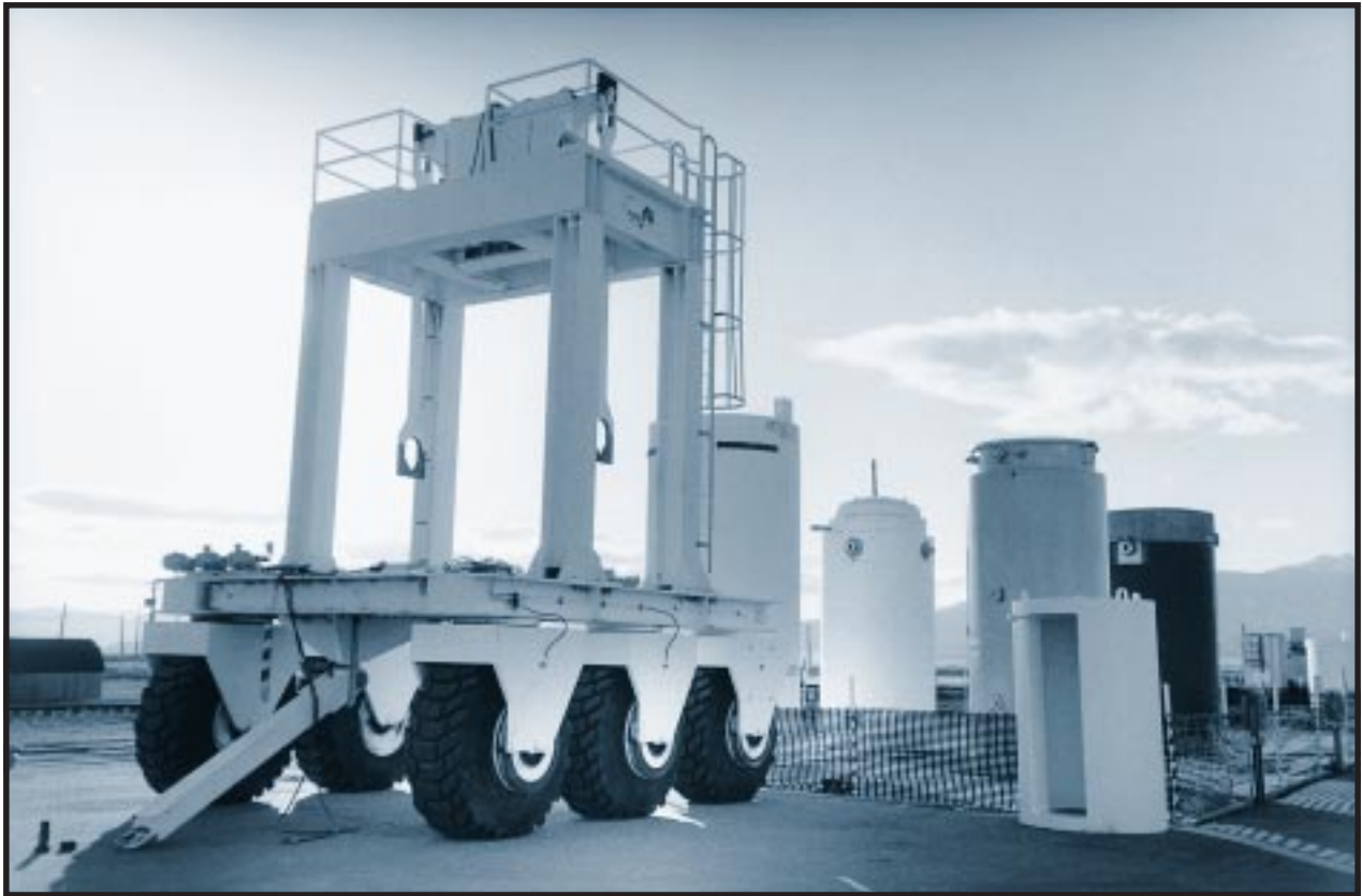
Straddle carrier for moving casks of spent fuel into dry storage. The Department of Energy is replacing underwater pool storage with these dry casks to increase safety and reduce costs. Idaho National Engineering Laboratory. March 17, 1994.
