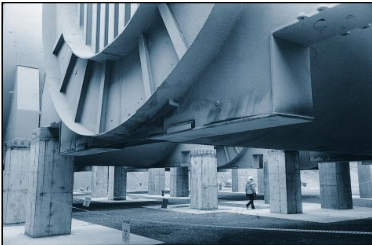
Use of the thick submarine hull as a disposal container provides extra isolation between the environment and the low-level waste and toxic lead that remain after the reactor fuel is removed. Trench 94, Hanford Site, Washington. December 20, 1993.
