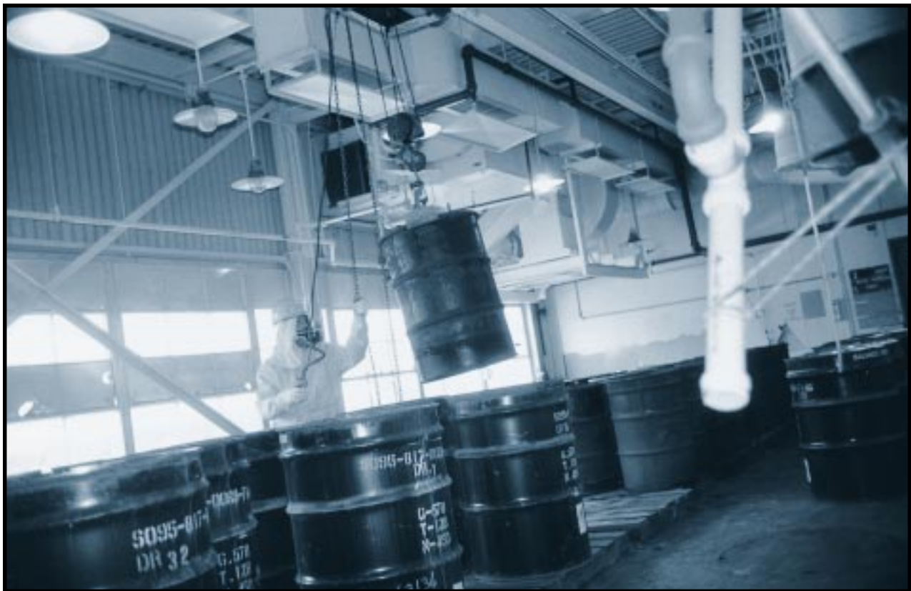
A Fernald worker overpacks rusting 55-gallon drums of low-level mixed waste by sealing them inside larger new 85-gallon drums. Some 50,000 deteriorating drums of Fernald waste stored outdoors for many years are being overpacked in a project that began in the late 1980s. Plant 5, formerly the Metals Production Plant, Fernald Environmental Management Project, Fernald, Ohio. December 28, 1993.
