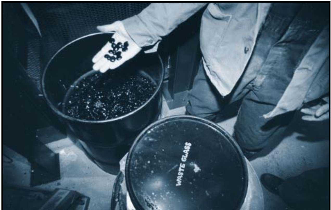
The vitrification of low-level mixed waste was demonstrated during the Minimum Additive Waste Stabilization pilot project. This demonstration used nonradioactive waste simulating soils and sludges contaminated with uranium and thorium. It produced several thousand kilograms of thumbnail-sized glass pebbles. This innovative technology makes wastes more stable while reducing waste volume and rendering them safer for disposal. MAWS Facility, Fernald Environmental Management Project, Fernald, Ohio. December 28, 1993.
