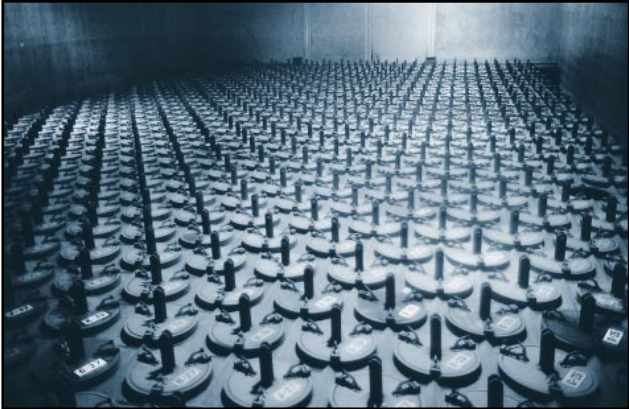
Irradiated nuclear fuel in dry storage. Building 603, Idaho Chemical Processing Plant, Idaho National Engineering Laboratory. March 17, 1994.
