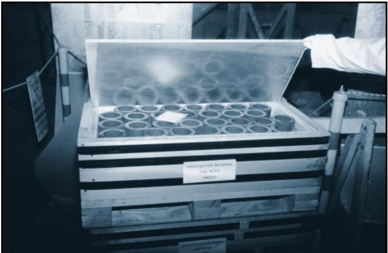
These Mark 31 depleted uranium target element inner cores are part of the Department's large inventory of nuclear materials left "in the pipeline" when the Cold War ended. These materials are no longer needed for their originally intended use. The Department will work with regulators and other interested parties to determine how materials like these should be managed. Plant 6, formerly the Metals Fabrication Plant, Fernald Environmental Management Project, Fernald, Ohio. December 28, 1993.
