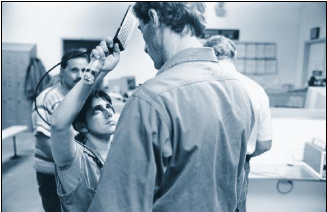
Health-physicist technician conducts a whole-body survey for potential radioactive contamination. She slowly moves a detection instrument over a worker, holding the meter within a quarter of an inch of his body. Plutonium Finishing Plant, Hanford Site, Washington. December 20, 1993.
