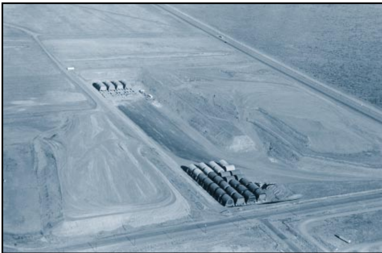
Hull sections of decommissioned nuclear-powered submarines are put in disposal trenches. The used nuclear fuel is removed from the sections of submarine hulls that contain nuclear reactors. The radioactively contaminated hull sections with the defueled reactors inside are then transported by barge to Hanford, where they are placed in a trench for burial. Trench 94, Hanford Site, Washington. July 12, 1994.
