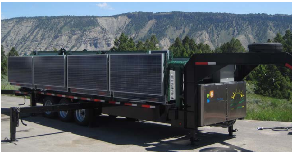
Figure 2. Mobile PV system shown stowed on the trailer upon delivery to Yellowstone National Park. Photo: Jim Evanoff
