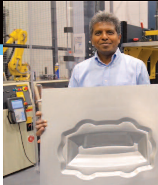
A computer program generates a tool path for the robots based on a CAD design, turning 2 D sheet metal into a 3 D part.
