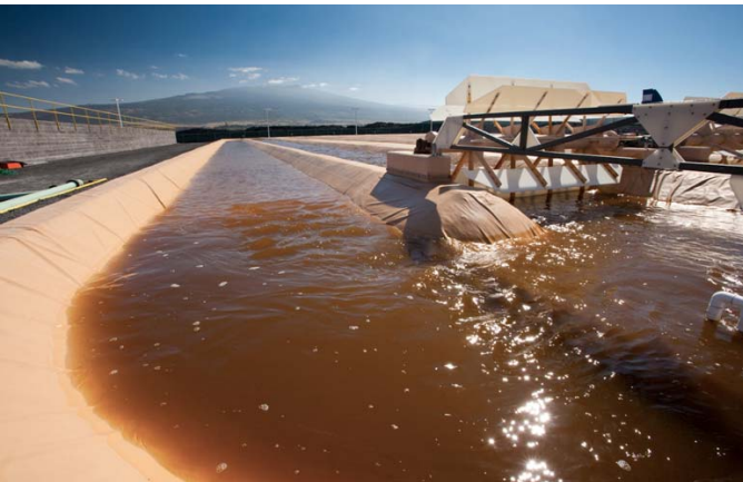
Raceway Pond- Cellana LLC, HI
