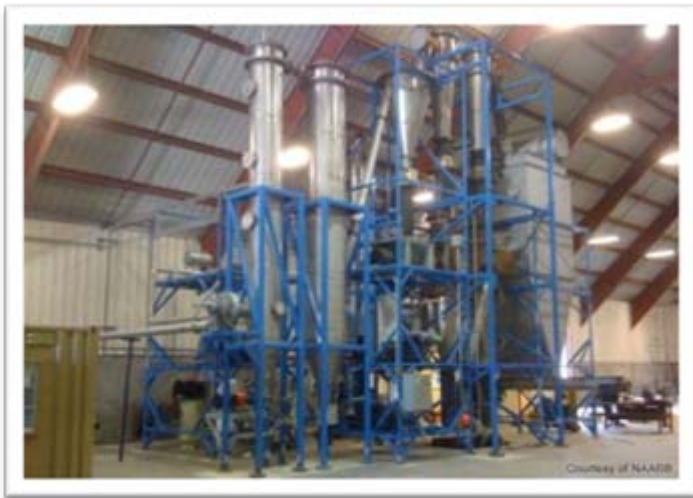
A gasifier being used by a NAABB partner to convert whole algal biomass to fuels
