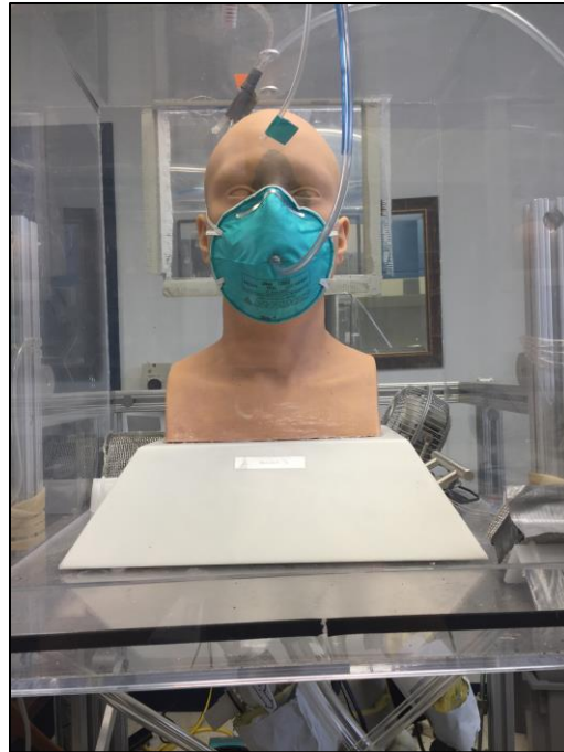
Figure 10. Fit Test Static Headform During Fit Test.
