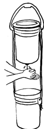
Figure 5: The Tap Up – a two bucket hand sink . Credit: Lippincott (2011), CERN Open Hardware Licence
