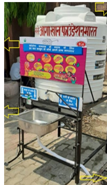
Figure 9: pedal operated handwashing station with large tank. Credit: Aga Khan Foundation, India
