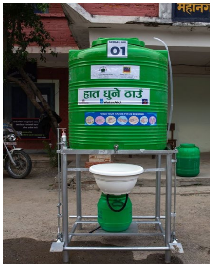
Figure 10: pedal-operated handwashing station with large tank. Credit: WaterAid Nepal
