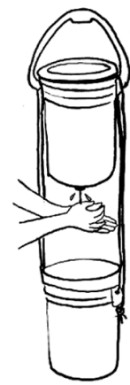
Figure 8: The Tap Up – a two bucket hand sink . Credit: Lippincott (2011), CERN Open Hardware Licence
