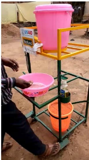
Figure 11: pedal-operated handwashing station. Credit: Tearfund DRC
