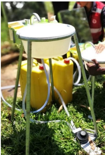
Figure 19: Jengu connected to jerry cans filled with water; variations of the Jengu handwashing device (left to right: for people with reduced mobility, children and adults) Credit: G. Rose, British Red Cross; Arup
