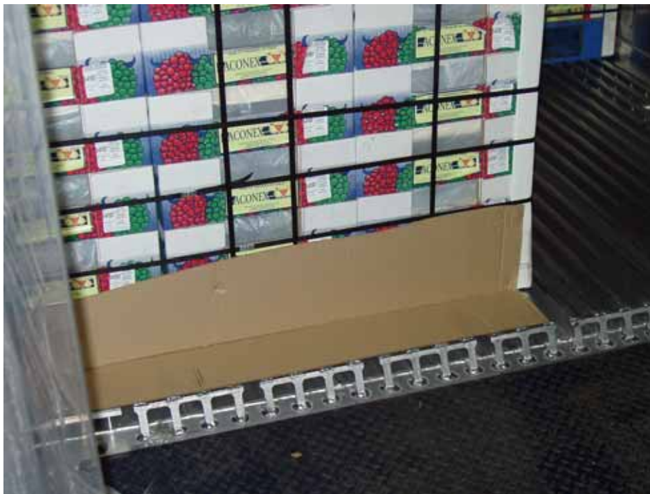
Figure 3-7-5 Proper placement of cardboard between the last pallet row of fruit and the back doors of the container
