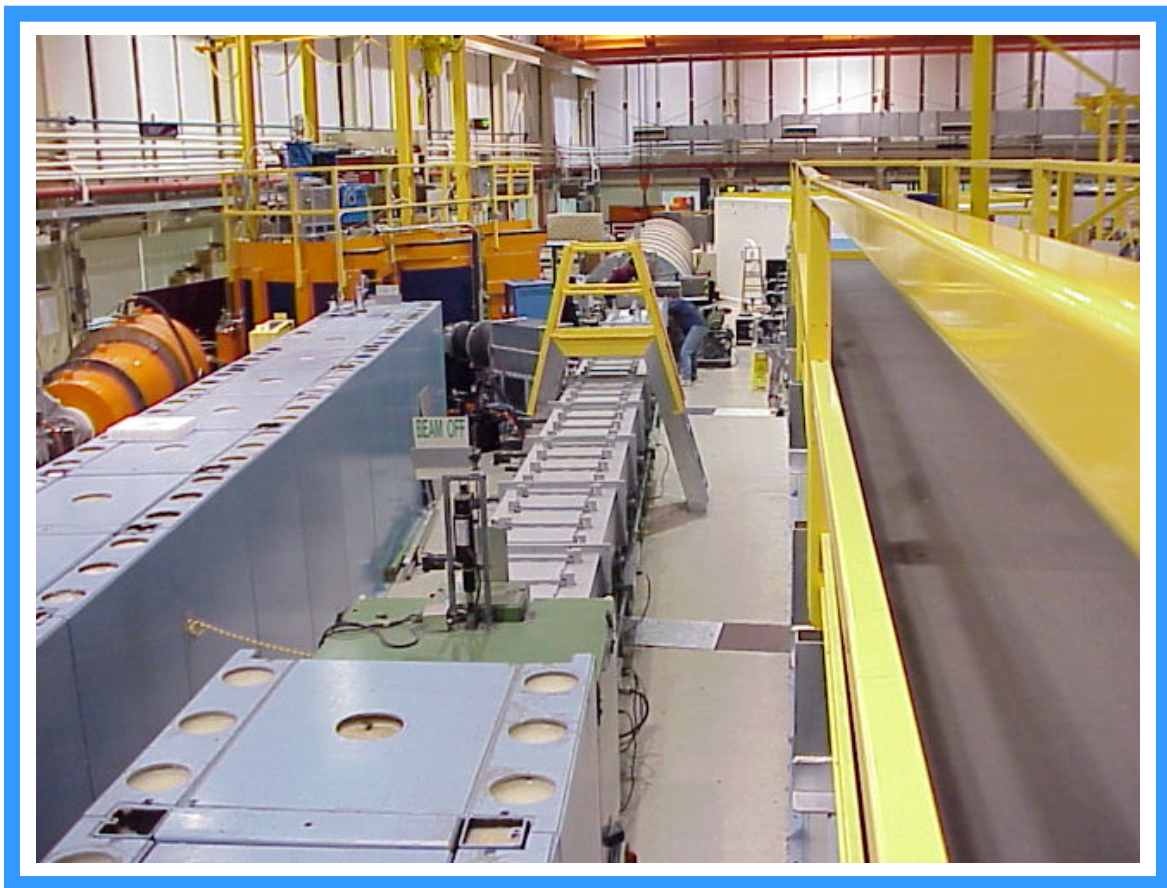
Figure 7: Photograph of the NG3 30 m SANS instrument. The picture was taken from the bridge walk just before the velocity selector shield.
