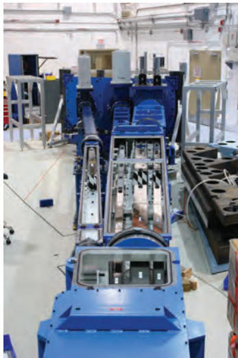
New guides assembled at various stages. Upper right: beam shutters partially installed at the C100 wall. Lower right: John Copley and Jeff Zeigler survey recently arrived guide components.
