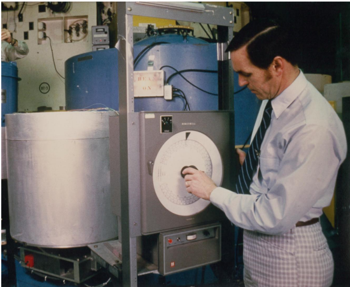
Dick Kelly preparing an experiment on the neutron spectroscopy of molecules bound on a catalyst, at the BT-4 Be-filter-analyzer spectrometer in 1981.
