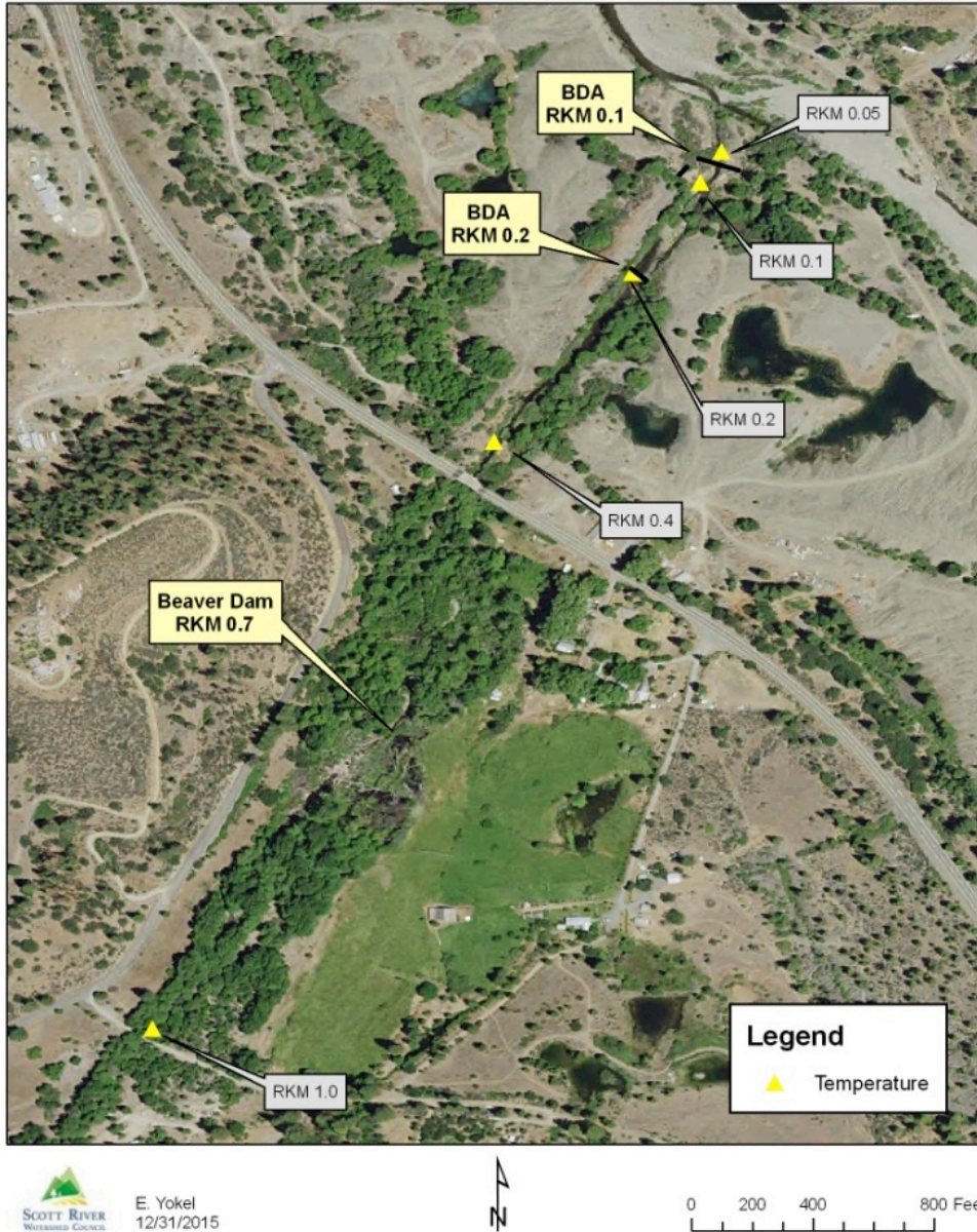
Figure 12. Location of surface water temperature monitoring stations in lower Sugar Creek, used in this study, in relation to the beaver dam analogues which were installed (thin black lines). Rkm = river kilometer, which refers to the distance upstream from the mouth of a river or creek.
