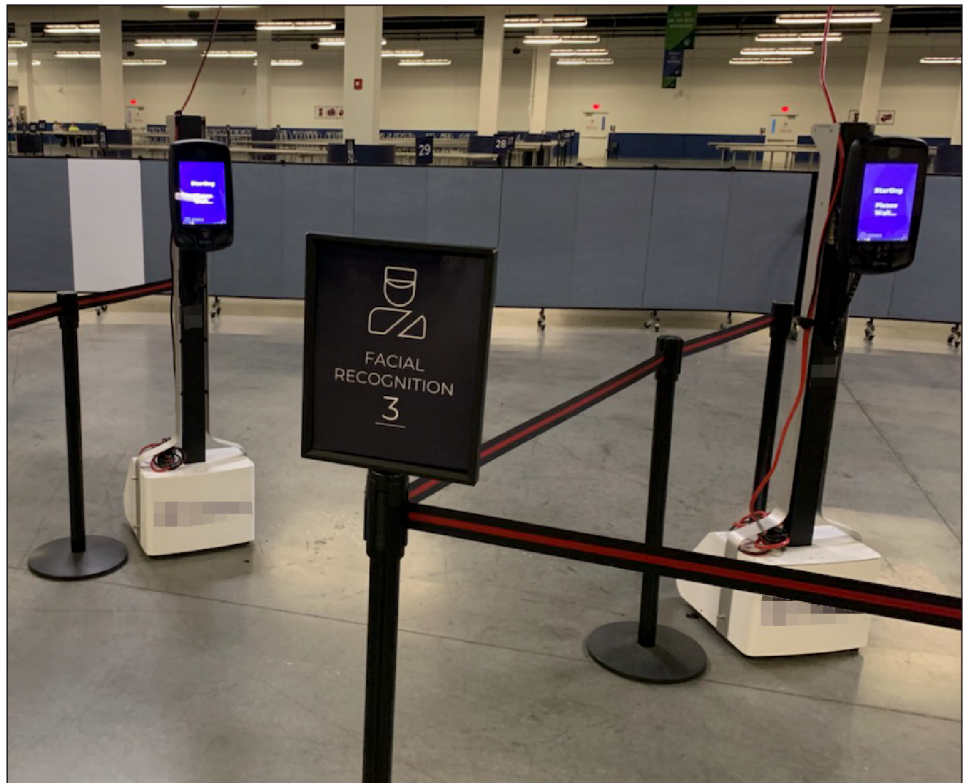
Figure 4: Example of Cameras and Display Screens Used for Facial Recognition at the Port Canaveral Seaport
