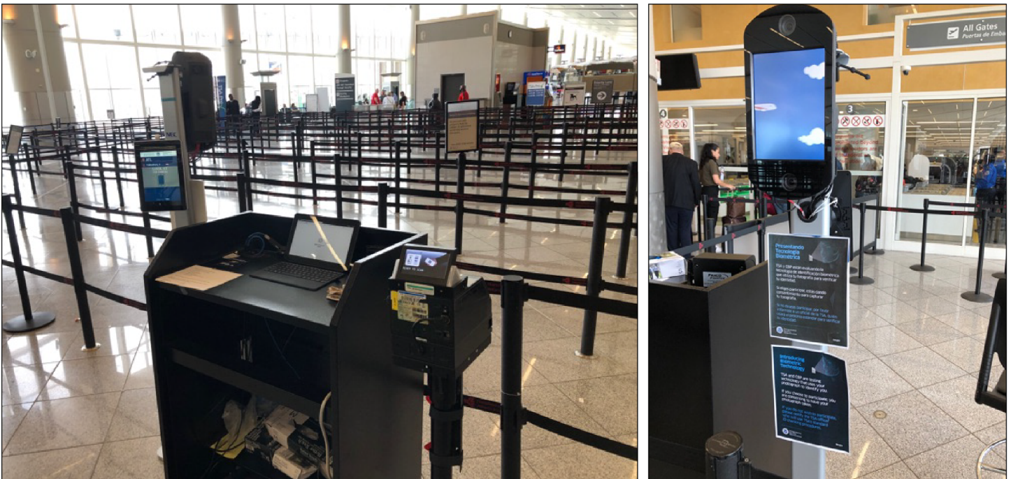
Figure 8: Facial Recognition Cameras Used for Facial Recognition during a Joint Transportation Security Administration and U.S. Customs and Border Protection Pilot Test at the Hartsfield-Jackson Atlanta International Airport
