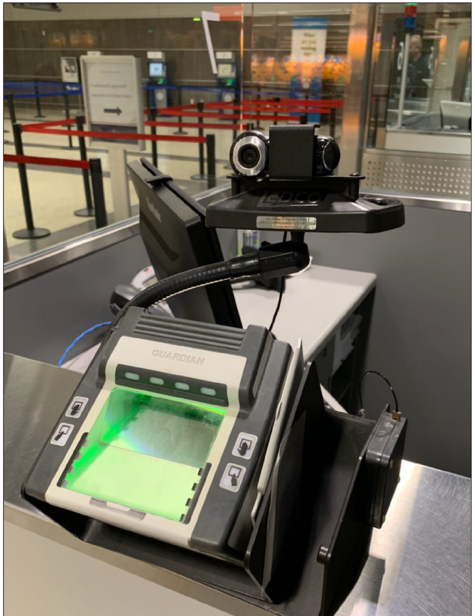
Figure 3: Example of a Camera Used for Air Entry Facial Recognition, Above a Fingerprint Scanner
