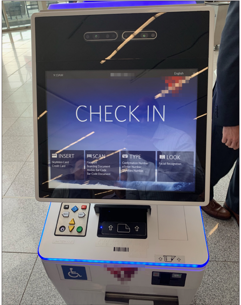
Figure 9: Delta Air Lines Check-in Kiosk at the Hartsfield-Jackson Atlanta International Airport That Provided Travelers with the Option to Participate In Facial Recognition Identity Verification during Self-service Check-in
