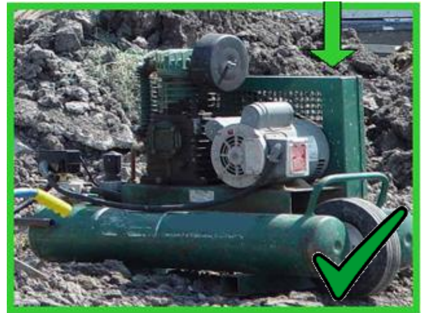
Guard Properly Installed
