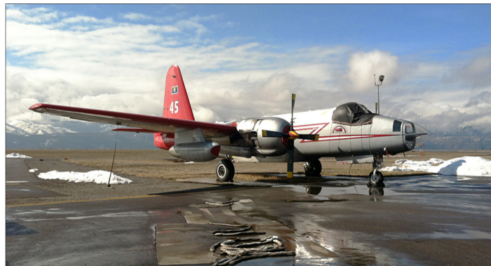
Korean War-era Lockheed P-2V Neptune owned by Neptune Aviation Services, originally a maritime patrol aircraft now converted to a large airtanker.
