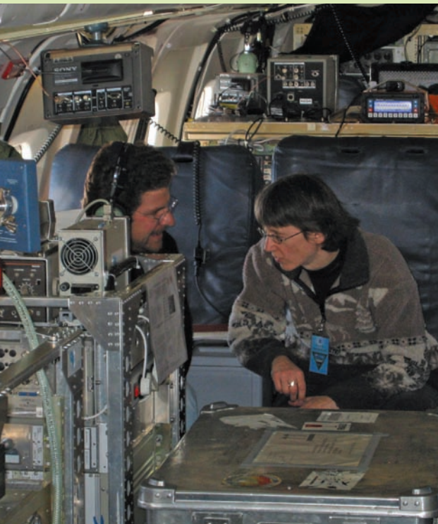
A typical DC-8 instrument setup where a scientist flies along with his or her instrument. Air sample tubes are mounted on the wings and in windows. MLS team member Michelle Santee talks with instrument scientist Armin Kleinböhl during a DC-8 flight.
