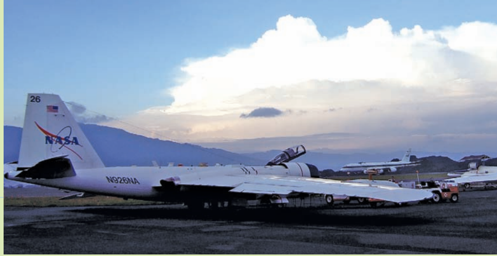
The WB-57 (above) and ER-2 (below) are high altitude aircraft, capable of flying into the lower stratosphere with a full payload of autonomously operated instruments.
