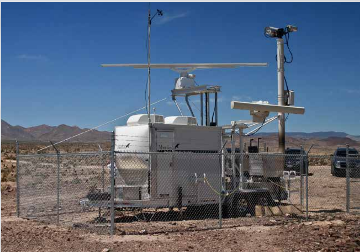
Merlin Radar System to track bird movements. Photo Credit: Eric Kershner.
