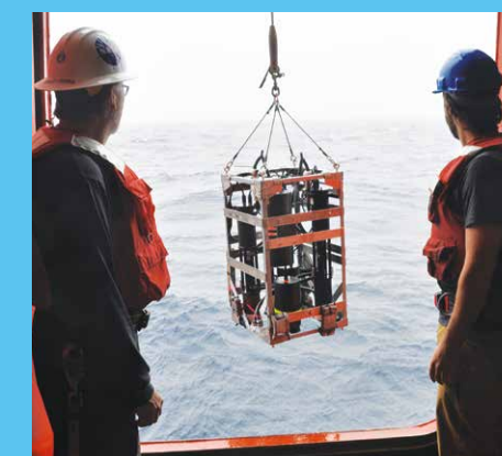
Ship-based optical instruments on ocean-going research vessels are often lowered into the water on a cable.
