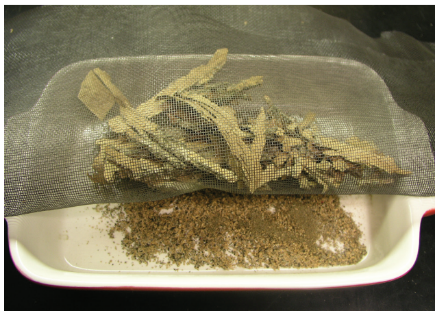
Figure 12. Sifting bark samples using standard nylon window screening. (Photo credit: Deborah Miller)
