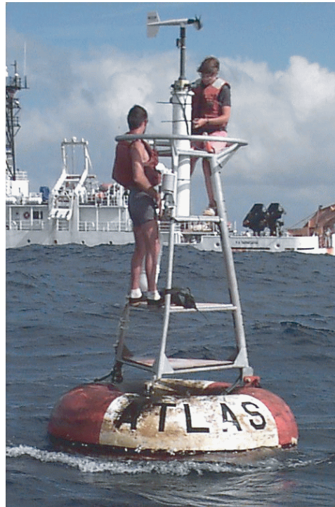
Figure 2: Repairing sensors on an ATLAS Mooring.
