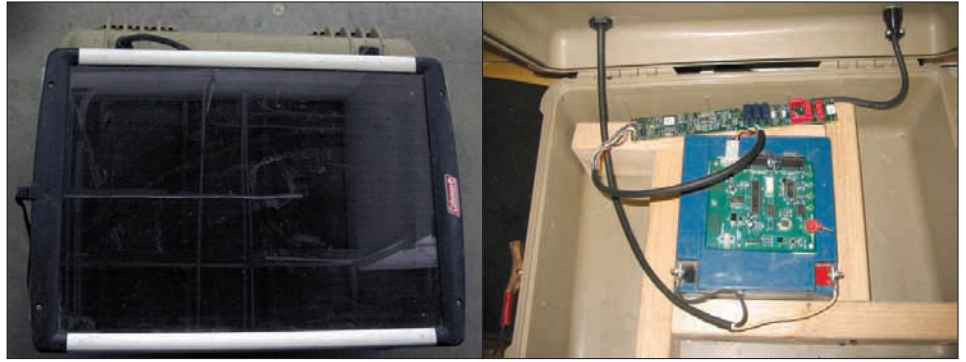
Figure 2. A remote passive integrated transponder (PIT) scanning unit built inside a 1520 Pelican™ case using an Allflex® scanner, a custom logger, a sealed lead acid battery, and a Coleman® model CL-600 solar charger.
