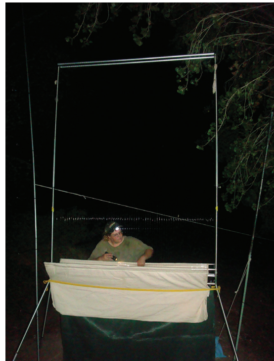
Figure 16. A harp trap set within a narrow opening at Cibola National Wildlife Refuge.
