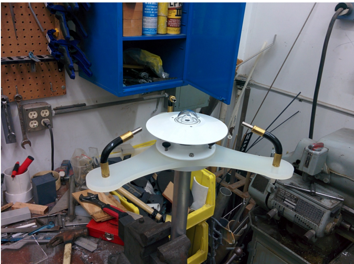
Photo of the prototype radiometer rinser. Fresh water is pumped from a large container and through each nozzle, rinsing the radiometer's glass dome.
