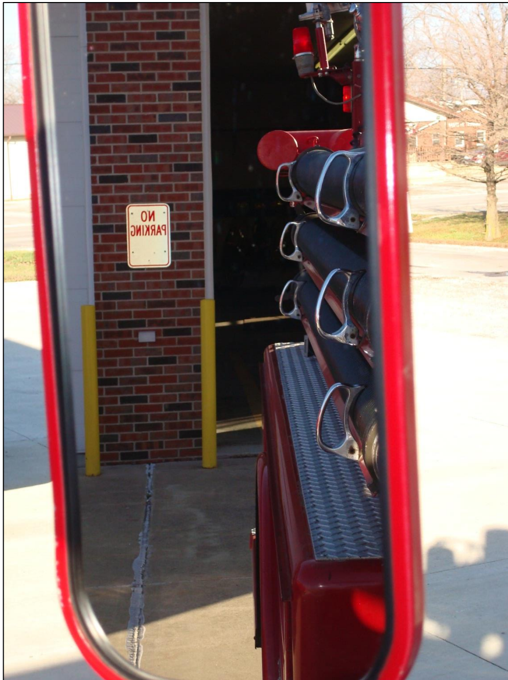
Photo 2. Photo of the driver side mirror on Brush Truck 12. Photo shows the narrow field of view that someone seated in the driver seat would typically see when using the driver side mirror to view the area behind and on the left side of the vehicle.
