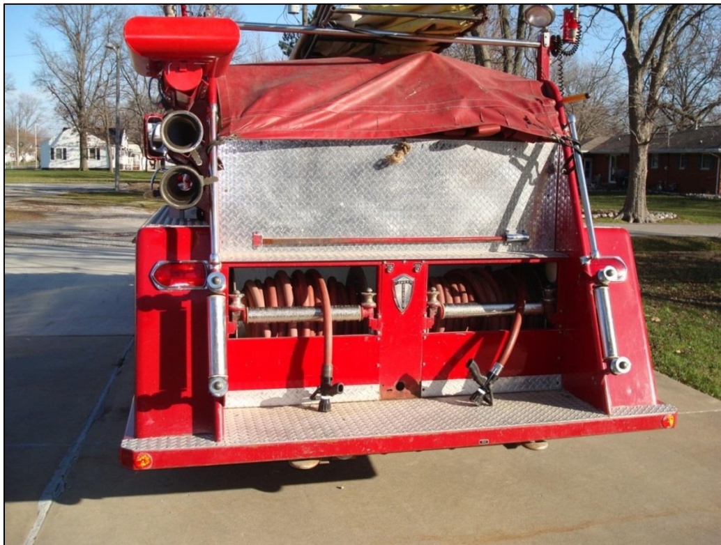
Photo 1. Rear of Brush Truck 12. Note hose reels mounted at the back of the apparatus. The victim likely intended to pull one of these hoses to use to combat the burning structure. (NIOSH photo)
