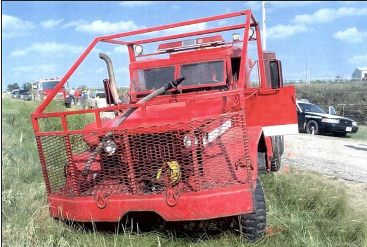
Photo 1. Front view of the front-bumper mounted platform
