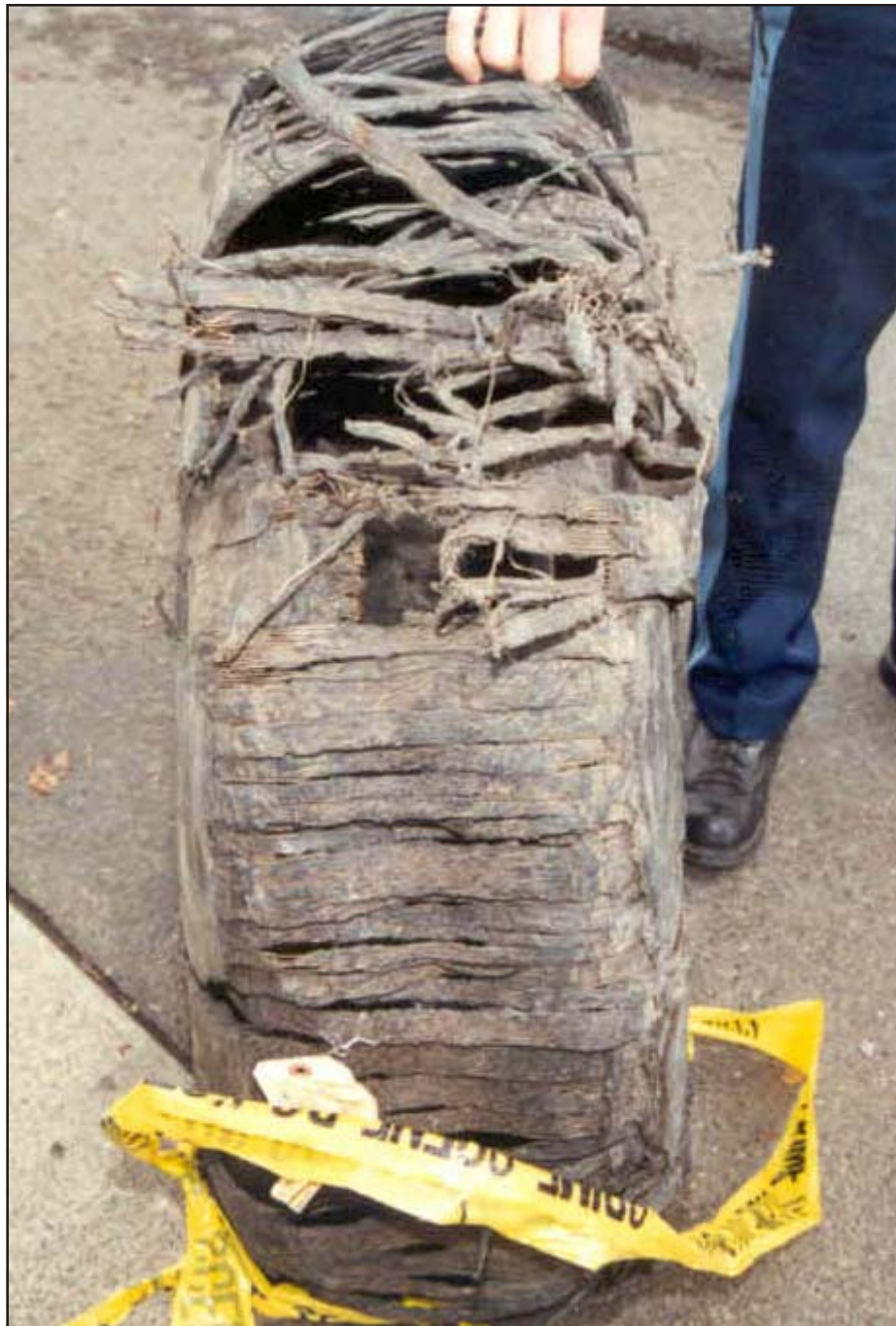
Photo 1. Tire That Experienced a Blowout on the Tanker Truck
