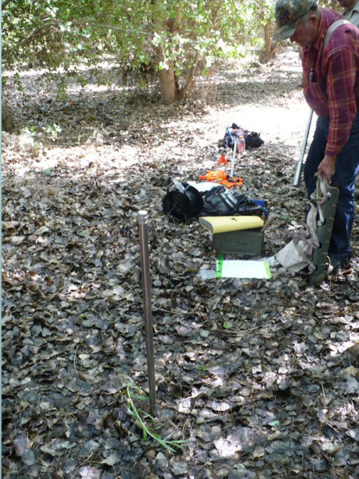
Piezometer near site center
