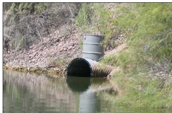
Figure C8b: Hoop net in culvert separates the backwater from the river. Tracking equipment inside the metal barrel is protected from damage by armor plating.
