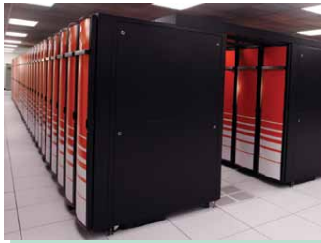
In 2006, ORNL's Cray XT3 and XT4 systems were combined and upgraded to quad-core processors. When the upgrades were complete, the new and improved Jaguar delivered a peak processing speed of 119 teraflops and 46 terabytes of aggregate memory.
