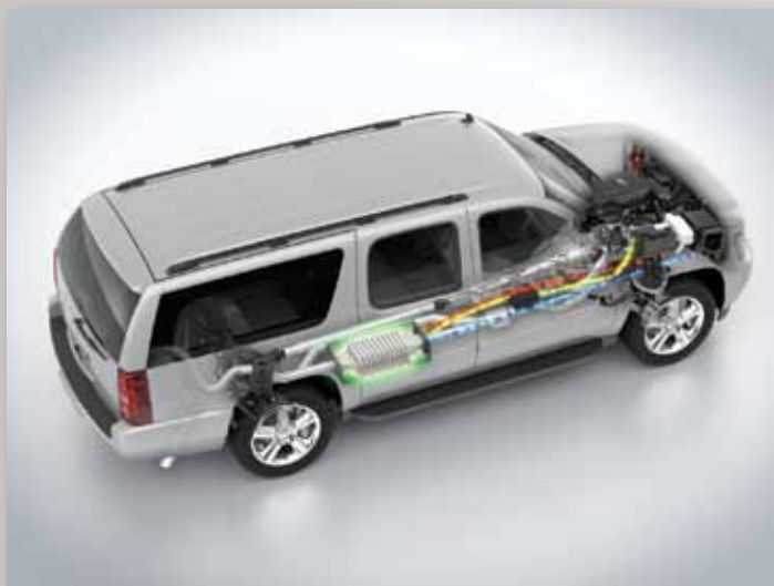
A thermoelectric generator in a Chevy Suburban would provide up to a 5 percent improvement in fuel economy. (Source: General Motors)
