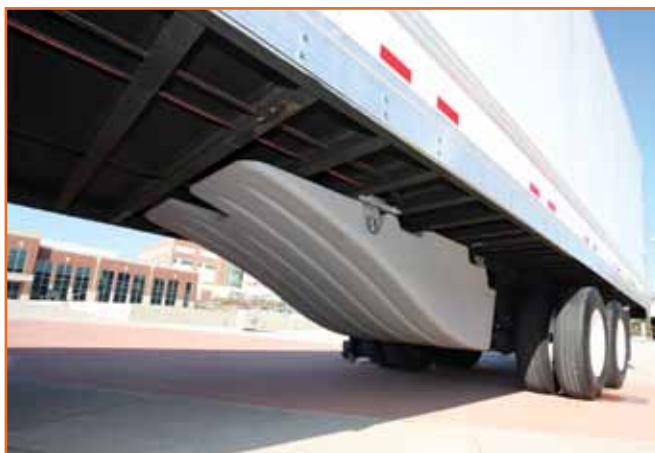
A trailer equipped with BMI Corp. SmartTruck UnderTray components.
