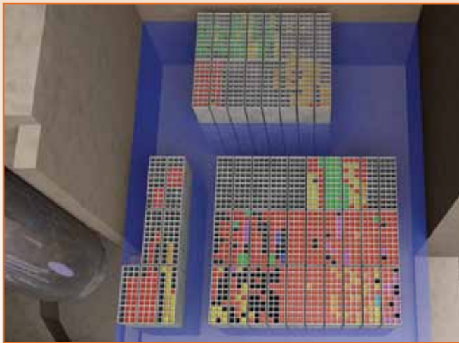
Rendering of the Fukushima reactor building spent fuel rod pool from above. The spent fuel rods are placed into one of three racks. The rods are colored by the date they are placed into the spent fuel pool.
