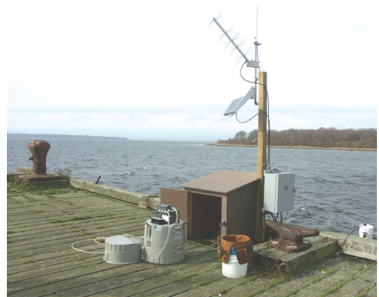
Figure 13.2. The System-Wide Monitoring Program at T-wharf on Prudence Island. Two water quality sondes are continuously deployed in PVC tubes extending into the Bay and data are transmitted near real time via telemetry. Nutrient and chlorophyll samples are also collected using the ISCO sampler shown here on the pier. Photo from NBNERR photo library.
