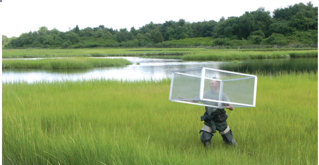
Figure 10.6. Using a throw trap to quantitatively sample nekton from salt marsh habitats. Photo from NBNERR photo library.
