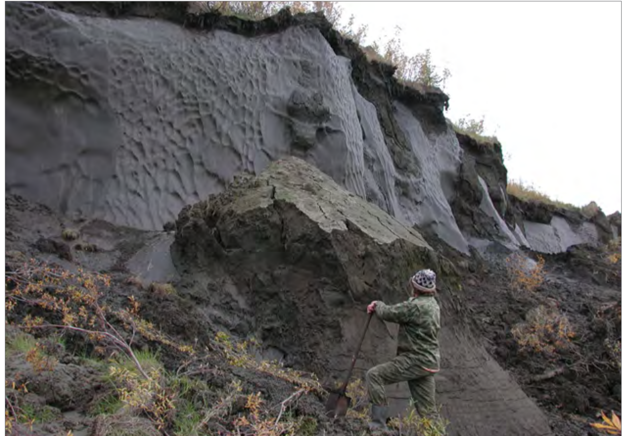
Sergey Zimov, director of the Northeast Science Station in Cherskii, Russia, stands near the base of this massive, exposed yedoma permafrost ice wedge, in this August 2001 photo taken at Duvanni Yar. The soil trapped behind the ice wedge is high in organic content, which could be released as carbon dioxide and methane if the yedoma thaws and rots. (Courtesy K. W. Anthony)
