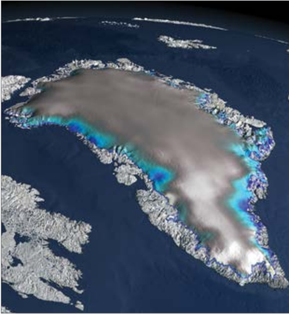
This visualization from the Ice, Cloud, and land Elevation Satellite (ICESat) shows changes in elevation over Greenland. ICESat's precise elevation change measurements, combined with other technologies, provide a comprehensive look at the behavior of Earth's ice sheets—critical for quantifying forecasts of sea level rise. Changes are shown between 2003 and 2006. White regions indicate a slight thickening, while blue shades indicate ice sheet thinning. Gray indicates no change in elevation. (Courtesy NASA Goddard Space Flight Center Scientific Visualization Studio)
